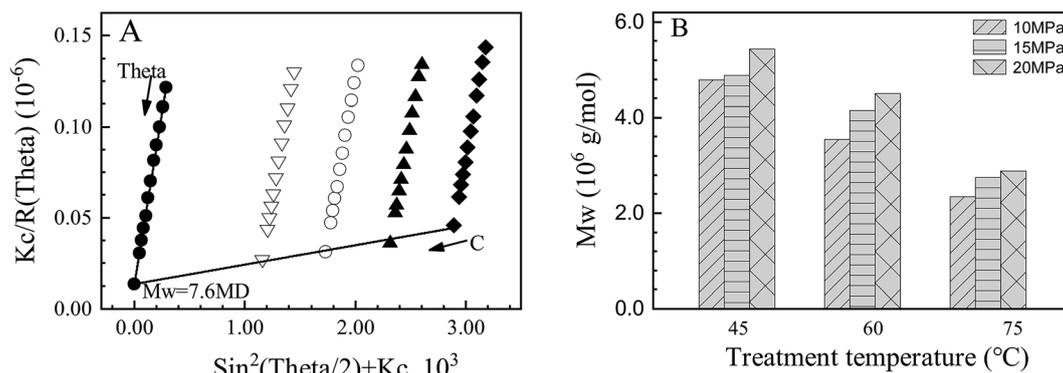
Fig. 1 The typical Zimm-plot of static light scattering data for HPAM in 1 mol L<sup>-1</sup> NaCl solution at concentrations of 0.04, 0.08, 0.12, 0.20 g L<sup>-1</sup> under 25.00 °C and molecular weight variations of HPAM after treatment of high temperature/pressure. (A) Represents the  $M_w$  of the control HPAM and (B) represents the  $M_w$  of the treated one.
