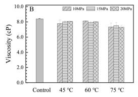
The HPAM hydrolysis degree and solution viscosity as a function of treatment temperature/pressure.
