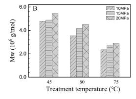
Fig. 1 The typical Zimm-plot of static light scattering data for HPAM in 1 moL L<sup>-1</sup> NaCl solution at concentrations of 0.04, 0.08, 0.12, 0.20 g L<sup>-1</sup> under 25.00 °C and molecular weight variations of HPAM after treatment of high temperature/pressure. (A) Represents the  $M_{\rm w}$  of the control HPAM and (B) represents the  $M_{\rm w}$  of the treated one.
