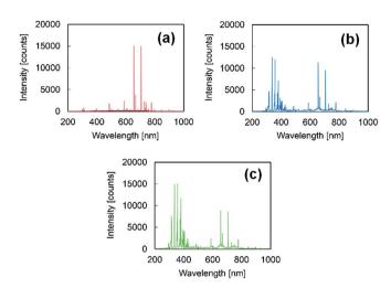
Fig. 1 OES spectra following HAP treatments in different air concentrations: (a) 0.01%, (b) 0.5%, and (c) 2.0%. Each measurement period was 3~s.
