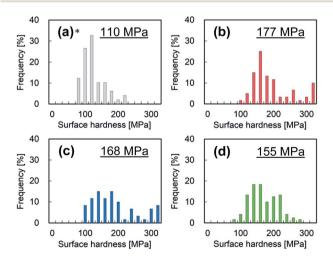
Fig. 7 Histograms of the surface hardness values of the PTFE samples without or with HAP treatments in different air concentrations: (a) asreceived (\*data measured in a previous study<sup>21</sup>), (b) HAP-treated in 0.01% air, (c) HAP-treated in 0.5% air, and (d) HAP-treated in 2.0% air. The underlined values denote the average surface hardness.
