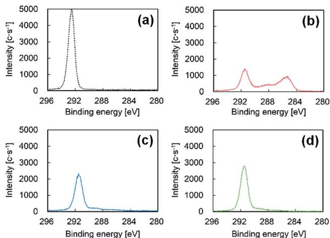
Fig. 4 C1s-XPS spectra of the PTFE samples without or with HAP treatments in different air concentrations: (a) as-received, (b) HAP-treated in 0.01% air, (c) HAP-treated in 0.5% air, and (d) HAP-treated in 2.0% air.
