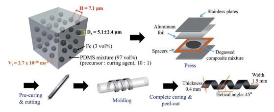
Fig. 1 Scheme for preparation of magnetically active helical soft robots via two-step polymerization method.
