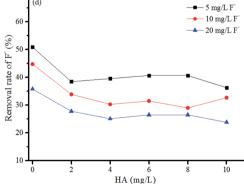
Fig. 7 The effects of co-substances on the removal rate of F<sup>-</sup>: (a) NO<sub>3</sub><sup>-</sup>, (b) SiO<sub>3</sub><sup>2-</sup>, (c) HCO<sub>3</sub><sup>-</sup>, and (d) HA. Experimental conditions:  $m=0.5~{\rm g~L^{-1}},~{\rm pH}=7.0~\pm~0.1,~{\rm and}~T=20~\pm~1~{\rm °C}.$
