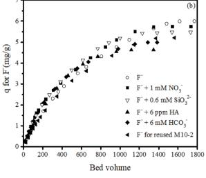
**Fig. 8** Filtration performance of fluoride with different fluoride-containing influent by M10-2: (a)  $F^-$  and  $Y^{3+}$  concentrations of permeate vs. bed volume and (b) accumulated q value vs. bed volume. Experimental conditions: pH =  $7.0 \pm 0.1$ , initial  $F^-$  concentration = 5.46 mg  $L^{-1}$ , pressure = 1.25 psi.
