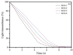
Fig. 3 Light transmittance curves of different casting solutions in different coagulation bath: (a) M2, (b) M6 and (c) M10 in different coagulation bath.
