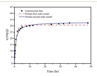
Fig. 6 Adsorption kinetics of F<sup>-</sup> on membrane M10-2: experimental data and pseudo-first order and pseudo-second order models. Experimental conditions:  $m=0.5~{\rm g~L^{-1}}$ , pH = 7.0  $\pm$  0.1, and  $T=20~{\pm}$
