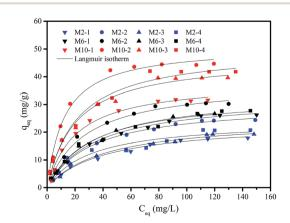
Fig. 4 Adsorption isotherm of F<sup>-</sup> by different membranes. Experimental conditions:  $m = 0.5 \text{ g L}^{-1}$ , pH = 7.0  $\pm$  0.1, reaction time = 48 h, and  $T = 20 \pm 1$  °C.
