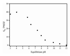
Fig. 5 Effect of equilibrium pH on adsorption of F $^-$  by membrane M10-2. Experimental conditions: m=0.5 g L $^{-1}$ , initial F $^-$  concentration = 21.26 mg L $^{-1}$ , and  $T=20\pm1$  °C.
