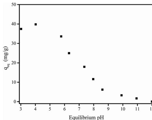
Fig. 5 Effect of equilibrium pH on adsorption of  $\text{F}^-$  by membrane M10-2. Experimental conditions:  $m = 0.5 \text{ g L}^{-1}$ , initial  $\text{F}^-$  concentration =  $21.26 \text{ mg L}^{-1}$ , and  $T = 20 \pm 1 \text{ }^\circ\text{C}$ .
