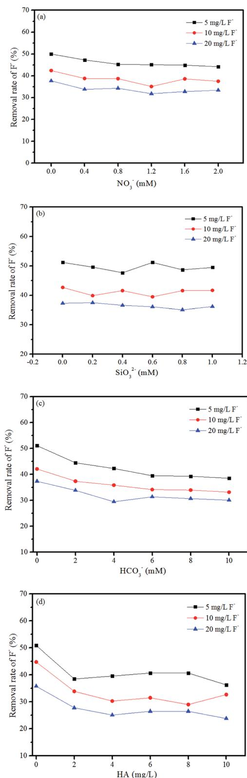
Fig. 7 The effects of co-substances on the removal rate of  $F^-$ : (a)  $NO_3^-$ , (b)  $SiO_3^{2-}$ , (c)  $HCO_3^-$ , and (d) HA. Experimental conditions:  $m = 0.5 \text{ g L}^{-1}$ ,  $pH = 7.0 \pm 0.1$ , and  $T = 20 \pm 1 \text{ }^\circ\text{C}$ .
