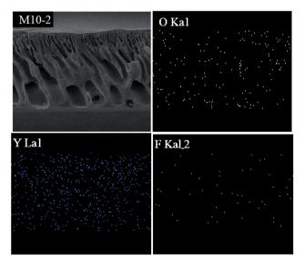
Fig. 9 EDS mapping of M10-2 after filtration.
