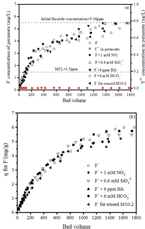
Fig. 8 Filtration performance of fluoride with different fluoride-containing influent by M10-2: (a)  $F^-$  and  $Y^{3+}$  concentrations of permeate vs. bed volume and (b) accumulated  $q$  value vs. bed volume. Experimental conditions:  $pH = 7.0 \pm 0.1$ , initial  $F^-$  concentration =  $5.46 \text{ mg L}^{-1}$ , pressure =  $1.25 \text{ psi}$ .
