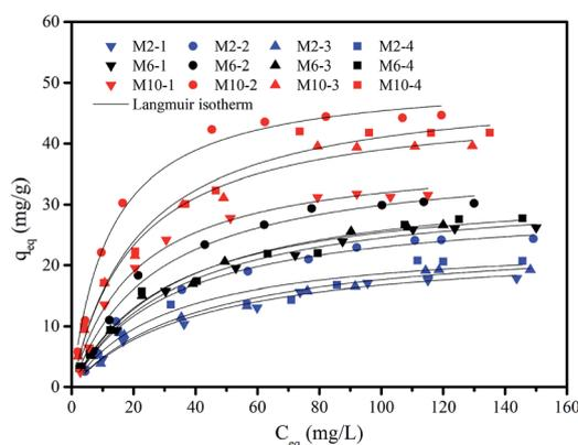
Fig. 4 Adsorption isotherm of F<sup>-</sup> by different membranes. Experimental conditions: *m* = 0.5 g L<sup>-1</sup>, pH = 7.0 ± 0.1, reaction time = 48 h, and *T* = 20 ± 1 °C.
