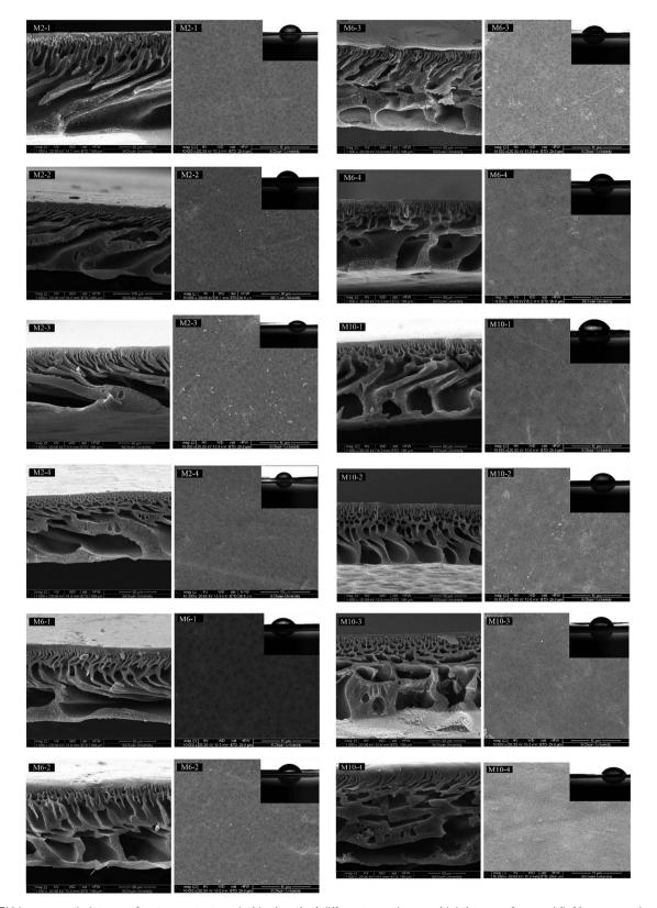
Fig. 2 SEM images and pictures of water contact angle (the inset) of different membranes: (right) top surface and (left) cross section.
