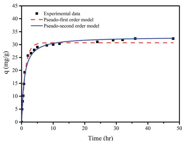
Fig. 6 Adsorption kinetics of F<sup>-</sup> on membrane M10-2: experimental data and pseudo-first order and pseudo-second order models. Experimental conditions:  $m = 0.5 \text{ g L}^{-1}$ ,  $\text{pH} = 7.0 \pm 0.1$ , and  $T = 20 \pm 1 \text{ }^\circ\text{C}$ .
