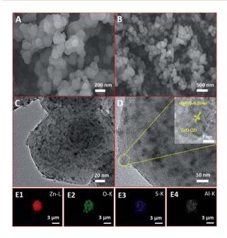
Fig. 2 (A) and (B) SEM images of AlR, ZnO@ZIF8-WL. (C) and (D) TEM images of AIR, ZnO@ZIF8-WL (the inset of (D) shows a HRTEM image of a ZnO QD, revealing a lattice spacing of 0.26 nm that arises from the (002) plane of the ZnO QD). (E1)-(E4) Elemental mapping of AlR,ZnO@ZIF8-WL
