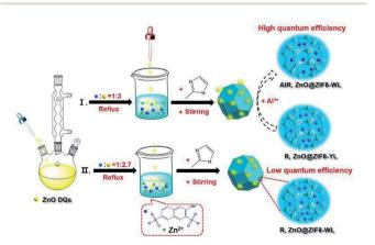
Fig. 1 Schematic of the synthesis process for the white light R,ZnO@ZIF8-WL, yellow light R,ZnO@ZIF8-YL, and in situ aluminium ions regulation for AlR, ZnO@ZIF8-WL
