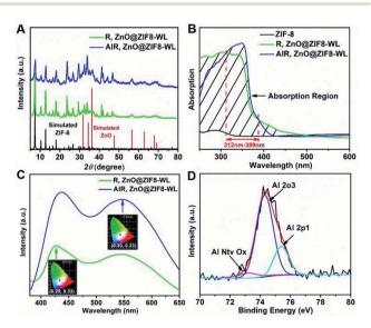
Fig. 3 (A) The PXRD of AIR,ZnO@ZIF8-WL and R,ZnO@ZIF8-WL. (B) The solid state UV absorption spectrum of AIR,ZnO@ZIF8-WL, R,ZnO@ZIF8-WL and ZIF-8, respectively. (C) The fluorescence spectrum of R,ZnO@ZIF8-WL and AIR,ZnO@ZIF8-WL at 356 nm. (Inset: the CIE coordinate diagram excited at 356 nm.) (D) XPS spectra of AIR,ZnO@ZIF8-WL.
