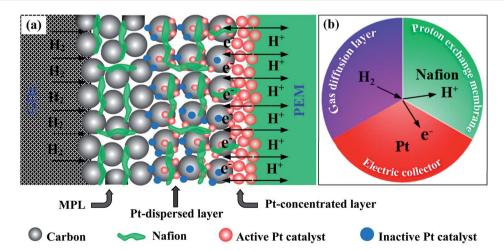
Fig. 6 (a) The advantages of DCL electrode for enhancing the pathways of  $H_2$ , electron, and proton; and TPB zones into the anodic catalyst structure in the DCL MEA. (b) Triple phase boundary simulation, where  $H_2$  (gas), Pt catalyst (solid), and Nafion (liquid) intersect.
