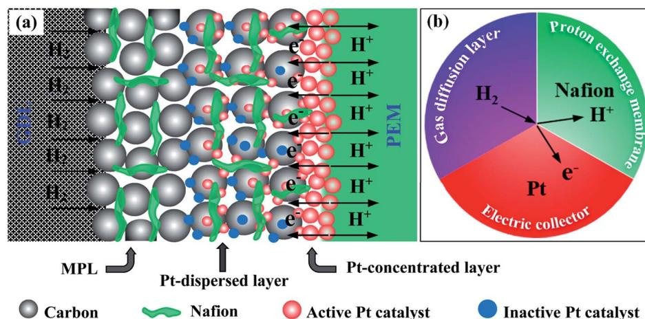
Fig. 6 (a) The advantages of DCL electrode for enhancing the pathways of H<sub>2</sub>, electron, and proton; and TPB zones into the anodic catalyst structure in the DCL MEA. (b) Triple phase boundary simulation, where H<sub>2</sub> (gas), Pt catalyst (solid), and Nafion (liquid) intersect.
