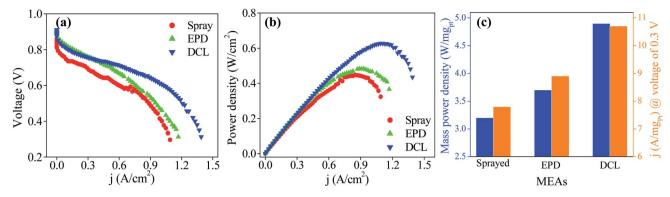
Fig. 5 (a) PEMFC polarization and (b) power density curves of MEAs consisting of spray, EPD, and DCL electrodes for anode sides, and cathode side is constantly spray electrodes, at working temperature of 80 °C, and (c) the corresponding mass power density and mass current density.
