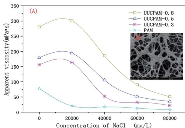
Fig. 13 Effect of the salt on the apparent viscosity of the UUCPAM polymer. (A) Apparent viscosity of UUCPAM in various salt concentrations and (B) SEM of UUCPAM in 20 000 mg L<sup>-1</sup> NaCl salt water.
