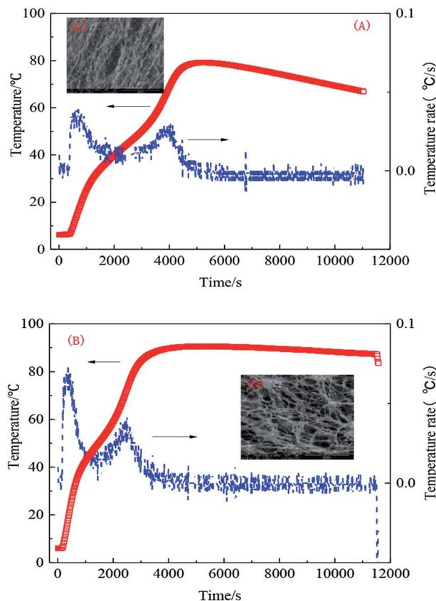
Fig. 6 Polymerization temperature changes with time. (A) 0.5 wt% UUC and (B) 1.0 wt% UUC; (C) SEM of sample A with 0.5 wt% UUC and (D) SEM of sample B with 1.0 wt% UUC.
