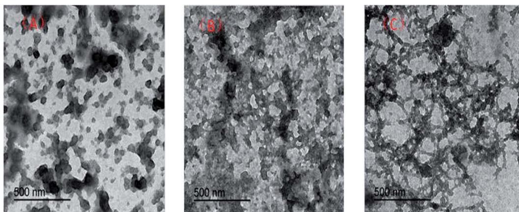
Fig. 4 TEM images of the hydrophobic associated polymer. (A) 0.1 wt% UUCPAM in 20 000 mg L<sup>-1</sup> NaCl salt water, (B) 0.2 wt% UUCPAM in 20 000 mg L<sup>-1</sup> NaCl salt water, and (C) 0.3 wt% UUCPAM in 20 000 mg L<sup>-1</sup> NaCl salt water.
