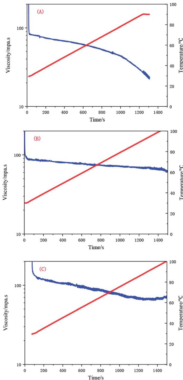
Fig. 15 Effect of temperature on the UUCPAM. (A) 0.1 wt% UUCPAM in 20 000 mg L<sup>-1</sup> NaCl salt water, (B) 0.2 wt% UUCPAM in 20 000 mg L<sup>-1</sup> NaCl salt water, and (C) 0.3 wt% UUCPAM in 20 000 mg L<sup>-1</sup> NaCl salt water.
