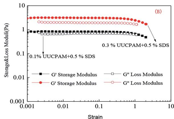
Fig. 9 Strain changes in the polymer viscoelasticity of different UUCPAM concentrations. (A) UUCPAM in 20 000 mg L<sup>-1</sup> NaCl solution and (B) UUCPAM + SDS in 20 000 mg L<sup>-1</sup> NaCl solution.
