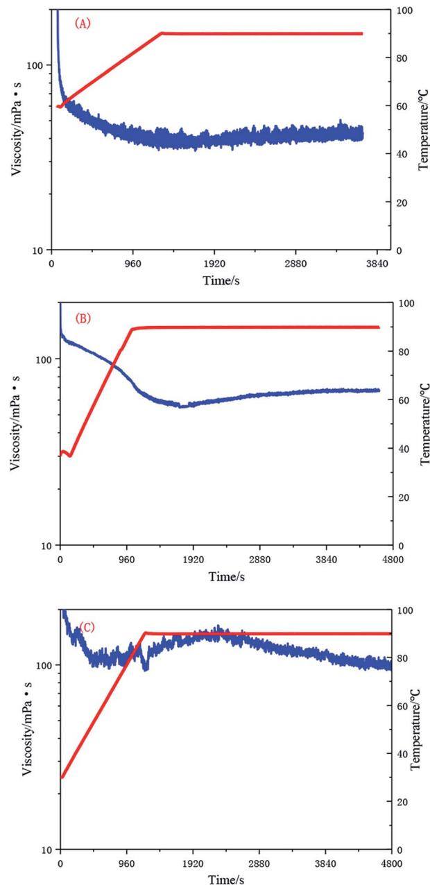
Fig. 16 Effect of the shear rate on the UUCPAM. (A) 0.1 wt% UUCPAM in 20 000 mg L<sup>-1</sup> NaCl water, (B) 0.2 wt% UUCPAM in 20 000 mg L<sup>-1</sup> NaCl salt water, and (C) 0.3 wt% UUCPAM in 20 000 mg L<sup>-1</sup> NaCl salt water.
