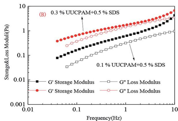
Fig. 10 Frequency changes in the polymer viscoelasticity in various UUCPAM concentrations. (A) UUCPAM in 20 000 mg L<sup>-1</sup> NaCl salt solution and (B) UUCPAM + SDS in 20 000 mg L<sup>-1</sup> NaCl salt solution.
