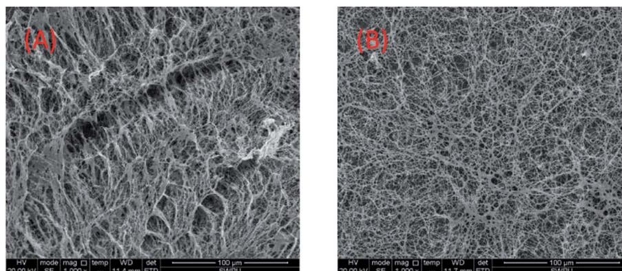
Fig. 14 SEM images of the UUCPAM polymer. (A) 0.3 wt% UUCPAM and (B) 0.3 wt% UUCPAM in 20 000 mg L<sup>-1</sup> NaCl salt water.
