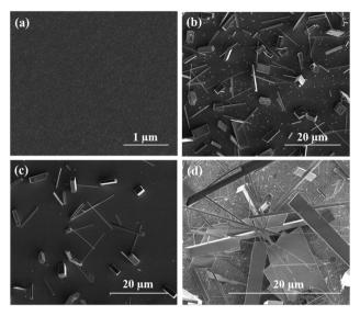
Fig. 5 The SEM images of the perovskite  $CH_3NH_3PbCl_3$  nanostructures grown at different reactive environments. (a) Room temperature without DMF in isopropanol solution, (b) 50  $\mu$ L DMF in 1 mL isopropanol solution, (c) 50  $\mu$ L DMSO in 1 mL isopropanol solution, and (d) 80 °C. The concentration of MACI/ISP solution was 6 mg mL $^{-1}$ .
