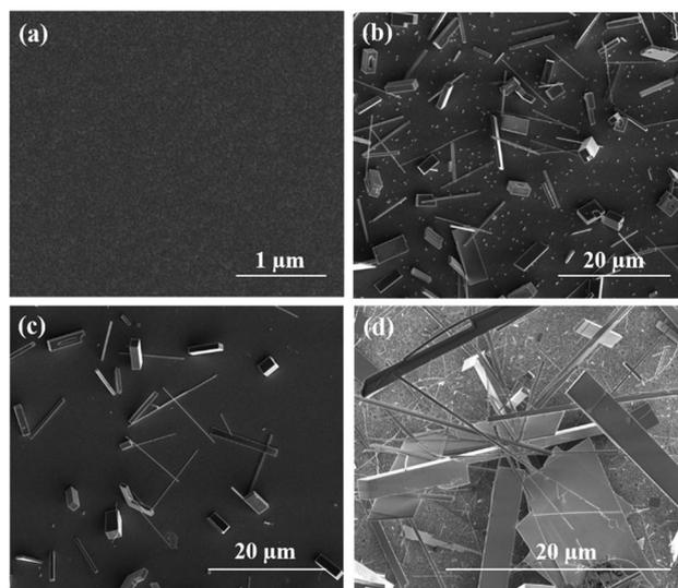
Fig. 5 The SEM images of the perovskite  $\text{CH}_3\text{NH}_3\text{PbCl}_3$  nanostructures grown at different reactive environments. (a) Room temperature without DMF in isopropanol solution, (b) 50  $\mu\text{L}$  DMF in 1 mL isopropanol solution, (c) 50  $\mu\text{L}$  DMSO in 1 mL isopropanol solution, and (d) 80  $^\circ\text{C}$ . The concentration of MAI/ISP solution was 6  $\text{mg mL}^{-1}$ .
