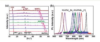
Fig. 6 (a) The PXRD patterns of the multiple compositional perovskite nanostructures grown at different halide ratios in the precursor solution. (b) Widely tunable fluorescence emission wavelength from the as-grown mixed halide perovskites.
