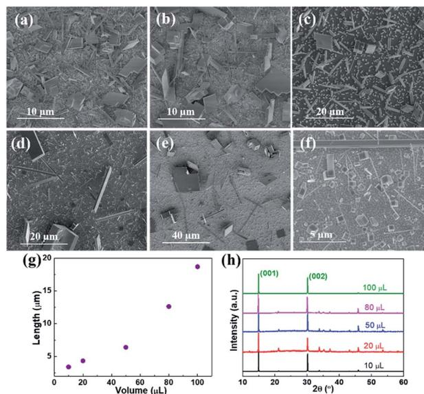
Fig. 2 The SEM images of the perovskite  $\text{CH}_3\text{NH}_3\text{PbBr}_3$  nanowires grown with different added volumes of DMF in 1 mL isopropanol. (a) 10  $\mu\text{L}$ , (b) 20  $\mu\text{L}$ , (c) 50  $\mu\text{L}$ , (d) 80  $\mu\text{L}$ , (e) 100  $\mu\text{L}$ , (f) the magnified image of a selected area in (e). (g) The corresponding length distributions and (h) PXRD patterns.
