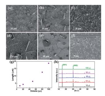
Fig. 2 The SEM images of the perovskite  $CH_3NH_3PbBr_3$  nanowires grown with different added volumes of DMF in 1 mL isopropanol. (a) 10  $\mu$ L, (b) 20  $\mu$ L, (c) 50  $\mu$ L, (d) 80  $\mu$ L, (e) 100  $\mu$ L, (f) the magnified image of a selected area in (e). (g) The corresponding length distributions and (h) PXRD patterns.
