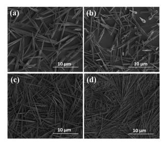
Fig. 4 The SEM images of perovskite  $CH_3NH_3Pbl_3$  nanowires (a) grown with 30  $\mu L$  DMF added into 1 mL isopropanol solution and (b) the corresponding samples after annealing at 100 °C for 15 minutes. The perovskite  $CH_3NH_3Pbl_3$  nanowires (c) grown with 10  $\mu L$  DMSO added into the isopropanol solution and (d) the corresponding samples after annealing at 100 °C for 15 minutes. The concentration of MAI/ISP solution was 10 mg mL $^{-1}$ .
