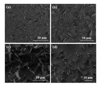
Fig. 1 The SEM images of perovskite  $CH_3NH_3PbBr_3$  nanostructures grown at different concentrations of  $CH_3NH_3Br$  in the isopropanol solution. (a)  $20 \text{ mg mL}^{-1}$ , (b)  $10 \text{ mg mL}^{-1}$ , (c)  $5 \text{ mg mL}^{-1}$ , (d)  $2 \text{ mg mL}^{-1}$ .
