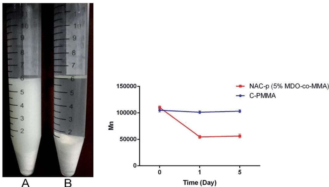
**Fig. 3** (Left) NAC-p (5% MDO-co-MMA) bone cement (A) and C-PMMA bone cement (B) soaked in glacial acetic acid for 24 h. (Right) GPC analysis of NAC-p (5% MDO-co-MMA) and C-PMMA.
