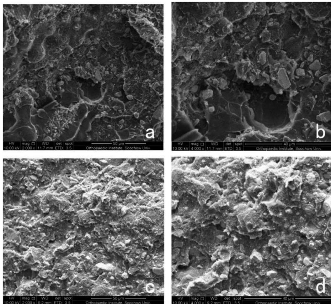
Fig. 4 Morphology of bone cement. SEM of sections of C-PMMA at 2000 $\times$  (a) and 4000 $\times$  (b) magnification and NAC-p (5% MDO-co-MMA) at 2000 $\times$  (c) and 4000 $\times$  (d) magnification.
