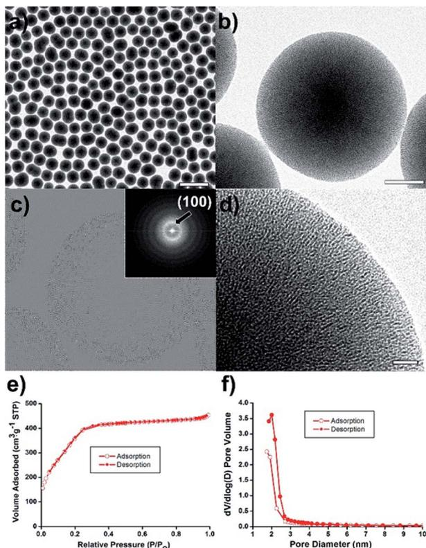
**Fig. 1** (a and b) TEM images, (c) FT pattern for (b) (inset of c) and IFFT image, (d) HRTEM image, (e)  $N_2$  adsorption/desorption isotherms, and (f) pore size distribution diagrams of  $mSiO_2$ . The bars represent 1  $\mu m$  (a), 100 nm (b), and 20 nm (d).
