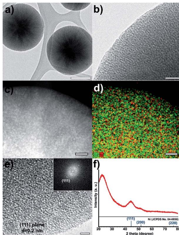
**Fig. 2** (a and b) TEM and (c) HAADF TEM images, (d) scanning TEM image with elemental mapping and (e) HRTEM images, and (f) XRD spectrum of  $Ni@mSiO_2$  nanostructure. The bars represent 200 nm (a), 20 nm (b–d), and 2 nm (e).
