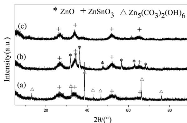
Fig. 1 XRD patterns of the precursor (a) before annealing, (b) after annealing at 500 °C for 3 h, and (c) corresponding calcined product washed with 20 wt%  $\text{NH}_4\text{Cl}$  solutions for 10 min.  $\text{ZnSnO}_3$ ,  $\text{Zn}_5(\text{CO}_3)_2(\text{OH})_6$ , and  $\text{ZnO}$  peaks are marked with plus sign, triangular symbol, and asterisks respectively.
