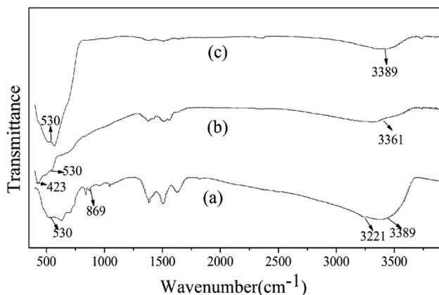
Fig. 3 FTIR data of the precursors (a) before annealing, (b) after annealing at  $500\text{ }^\circ\text{C}$  for 3 h, and (c) corresponding calcined product washed with 20 wt%  $\text{NH}_4\text{Cl}$  solutions for 10 min.
