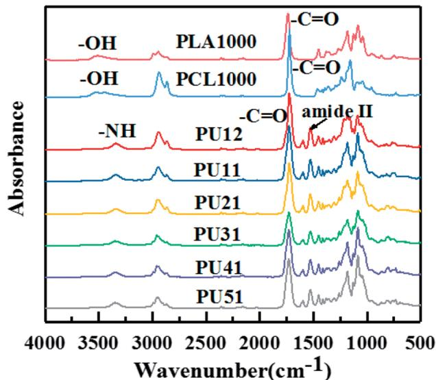
Fig. 1 FTIR spectra of the obtained bio-PU.
