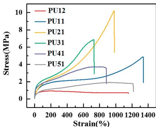
Fig. 3 Stress–strain curves of the obtained bio-PU.
