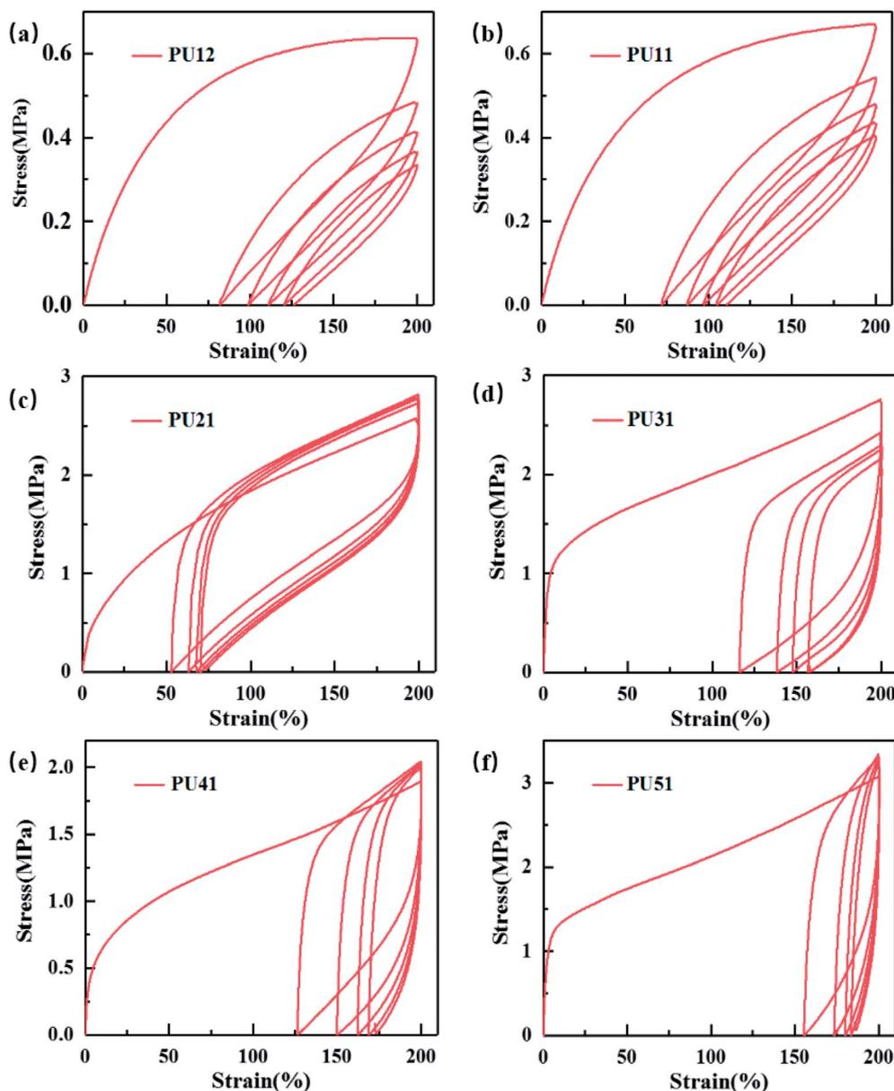
Fig. 4 Cyclic stress–strain curves of the obtained bio-PU.
