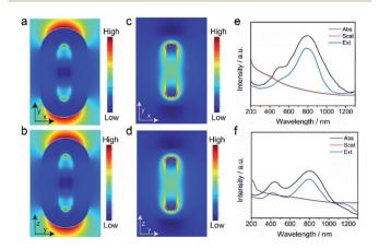
Fig. 4 Theoretical calculation of the EM filed of the AuNR@IR780/DOX (a and b) and AuNR (c and d), and absorption, scattering and extinction spectra of AuNR@IR780/DOX (e) and AuNR (f).
