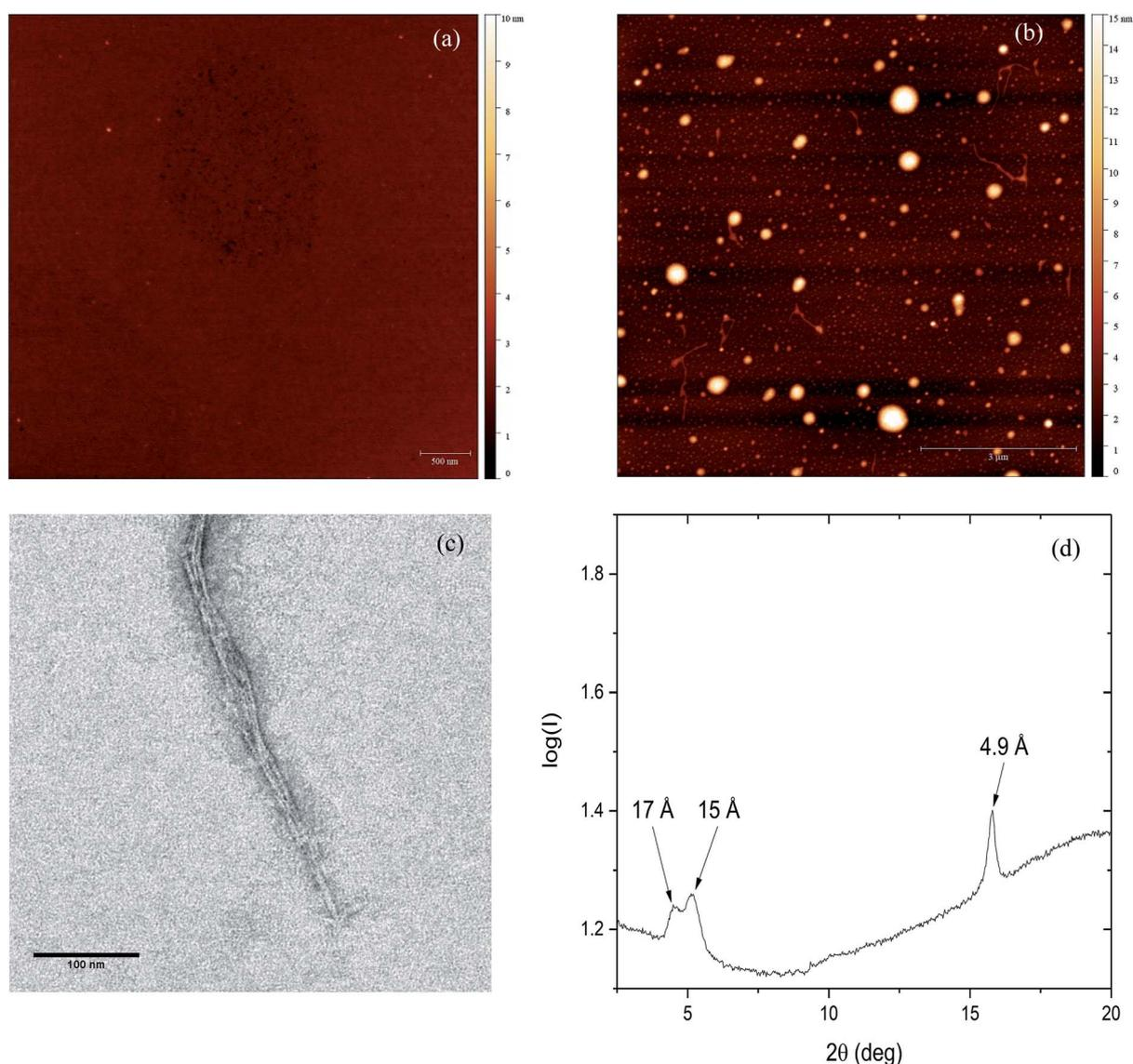
**Fig. 3** (a) AFM micrograph of monomeric PrP<sup>58–93</sup> peptide. (b) AFM micrograph of formed PrP<sup>58–93</sup> fibrils and oligomers in presence of ZnCl<sub>2</sub>. (c) TEM image of PrP<sup>58–93</sup> fibrils formed in presence of ZnCl<sub>2</sub>. (d) X-ray diffraction pattern for PrP<sup>58–93</sup> fibrils formed in presence of ZnCl<sub>2</sub>. Three reflections are visible: one meridional at 4.9 Å and two equatorial at  $\sim$ 15 Å and  $\sim$ 17 Å.
