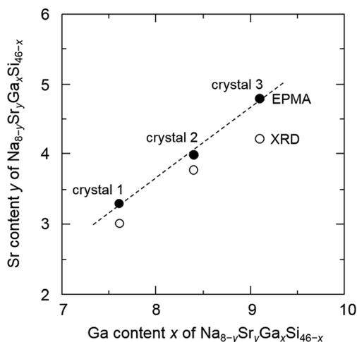
Fig. 2 Sr content (*y*) versus Ga content (*x*) of Na<sub>8-y</sub>Sr<sub>y</sub>Ga<sub>x</sub>Si<sub>46-x</sub>.
