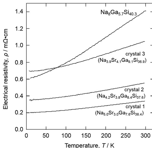
Fig. 4 Temperature dependence of the electrical resistivity of crystal 1 (Na<sub>5.0</sub>Sr<sub>3.0</sub>Ga<sub>7.6</sub>Si<sub>38.4</sub>), crystal 2 (Na<sub>4.2</sub>Sr<sub>3.8</sub>Ga<sub>8.4</sub>Si<sub>37.6</sub>), crystal 3 (Na<sub>3.9</sub>-Sr<sub>4.1</sub>Ga<sub>9.1</sub>Si<sub>36.9</sub>), and Na<sub>8</sub>Ga<sub>5.7</sub>Si<sub>40.3</sub>.<sup>12</sup>
