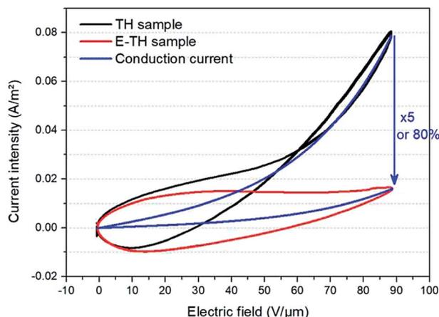
Fig. 7 Current versus electric field for unipolar sinusoidal voltages. Black and red lines refer to experimental measurement of the TH-sample and E-TH sample, respectively. Blue curves represent the conduction current component modelled by eqn (3).
