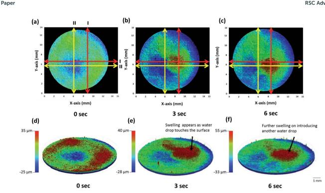
2D (a-c) and 3D (d-f) stitched images of whole matrix tablet surface with respect to time showing surface swelling and dissolution.
