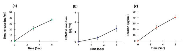
Fig. 15 (a) Drug release, (b) HPMC dissolution and (c) overall erosion profiles from the surface of matrix tablet.
