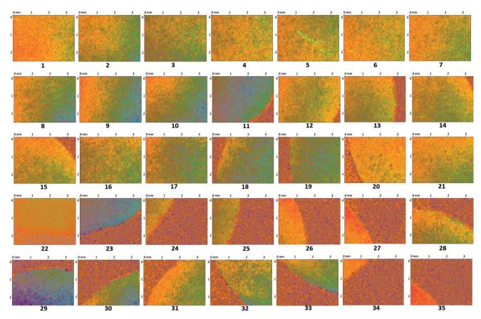
2D surface texture images (1-35) of the matrix tablet surface at time zero
