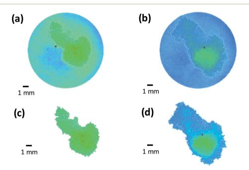
Fig. 12 Multiple regional analysis of surface swelling of matrix tablet using (a and b) image subtraction (c and d) image thresholding algorithm.
