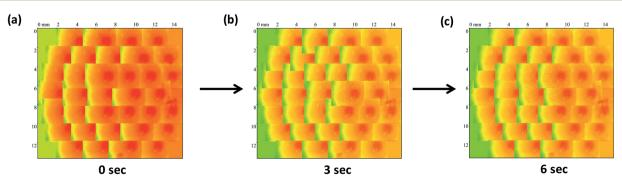
Fig. 7 The stitched images of matrix tablet surface at time points (a) 0 s, (b) 3 s and (c) 6 s after addition of liquid.
