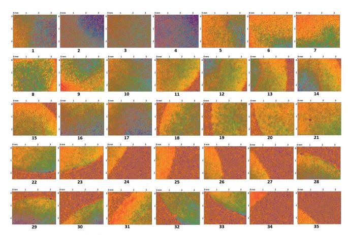
2D surface texture images (1-35) of the matrix tablet surface after 3 seconds
