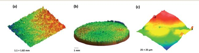
Fig. 9 3D surface texture images of HPMC matrix tablet (a) single image captured using Contour GT Elite K (b) stitched image developed using multiple images captured using Contour GT Elite K and (c) single image captured using AFM.
