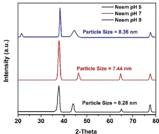
Fig. 3 XRD results of AgNPs using NE (pH 5, 7, 9).
