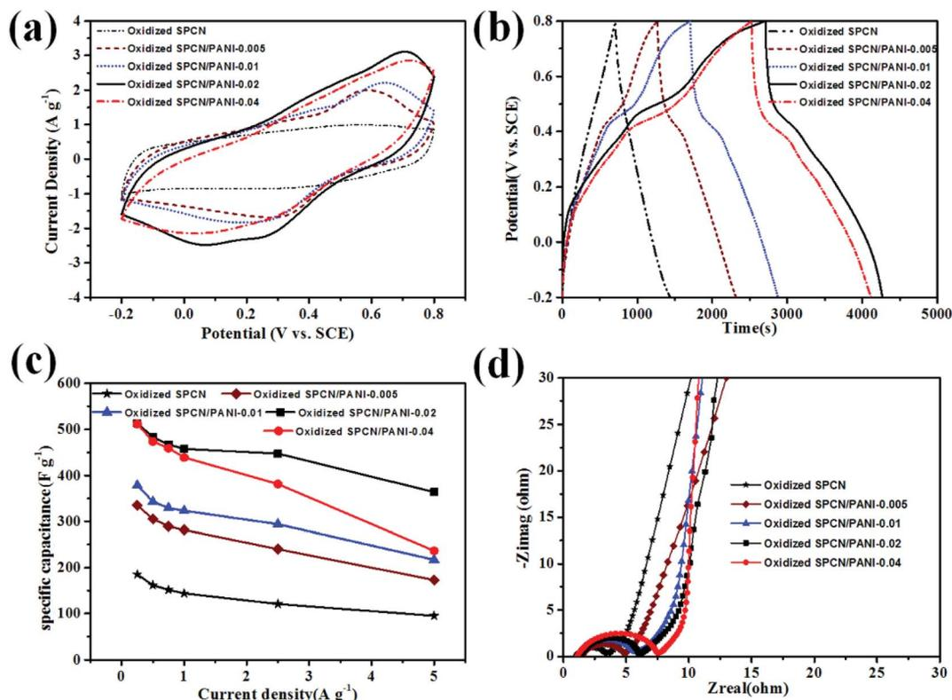
Fig. 4 (a) CV curves at the scan rate of  $5 \text{ mV s}^{-1}$  and (b) GCD curves at current density of  $0.25 \text{ A g}^{-1}$  of oxidized SPCN and oxidized SPCN/PANI-X; (c) specific capacitance versus current density and (d) Nyquist plots of oxidized SPCN and oxidized SPCN/PANI-X.
