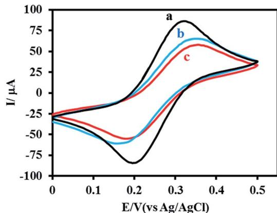
Fig. 3 Cyclic voltammograms of 0.5 mM of  $[\text{Fe}(\text{CN})_6]^{3-/4-}$  in 0.1 M PBS, pH 5.5, containing 0.1 M KCl at a scan rate of  $50 \text{ mV s}^{-1}$  obtained for electrodes at different assembly steps: flat gold (a), NPG (b) and aptamer functionalized NPG electrode before (c) and after immobilization with DHBA redox probe.
