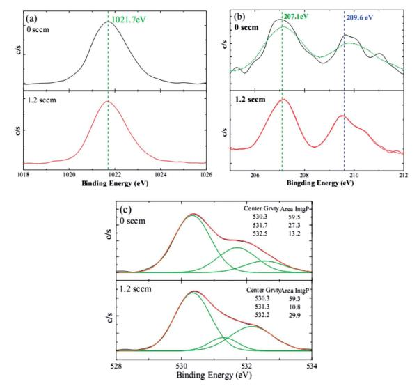
Fig. 4 The typical XPS spectra of (a) Zn 2p, (b) Nb 3d, and (c) O 1s of the NZO films with and without H doping.
