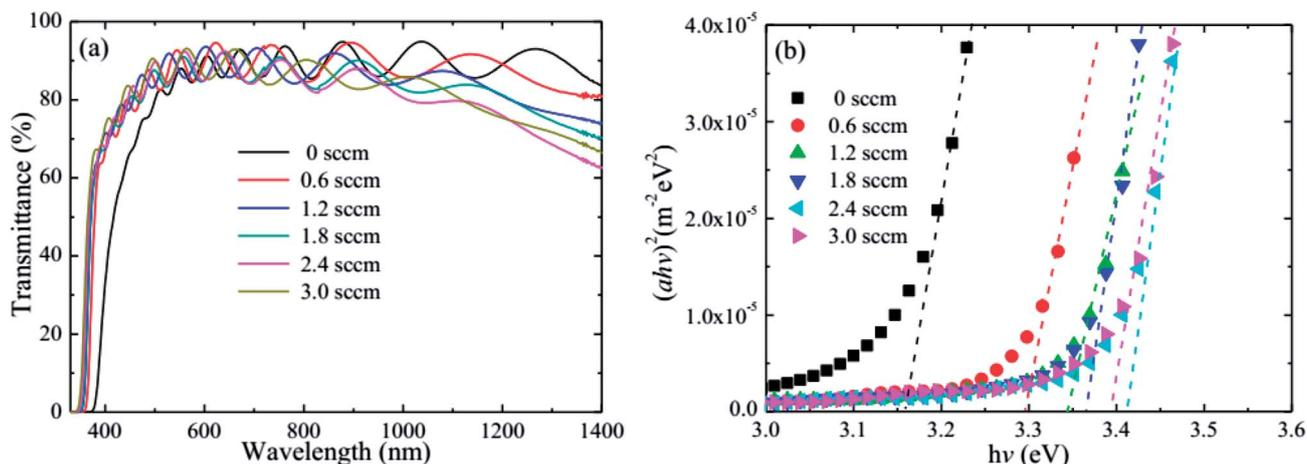
Fig. 6 (a) The optical transmittance, and (b) optical band gap of the HNZO films as a function of the flow rate of H<sub>2</sub>.
