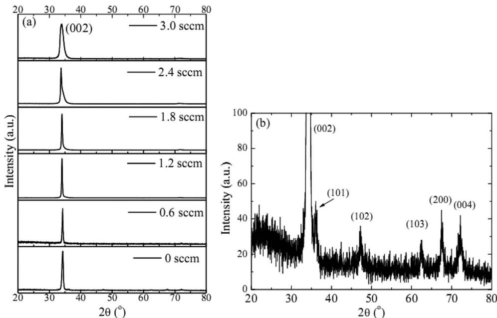
Fig. 2 (a) The XRD patterns of the HNZO films as a function of the flow rate of H<sub>2</sub>. (b) the amplified XRD pattern of the NZO film (0 sccm of H<sub>2</sub>).
