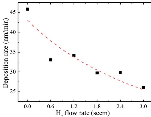
Fig. 1 The deposition rate of the HNZO films as a function of the flow rate of H<sub>2</sub>.
