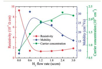
Fig. 5 The carrier concentration (n), mobility ( $\mu$ ), and resistivity ( $\rho$ ) of the HNZO films as functions of the flow rate of H<sub>2</sub>.
