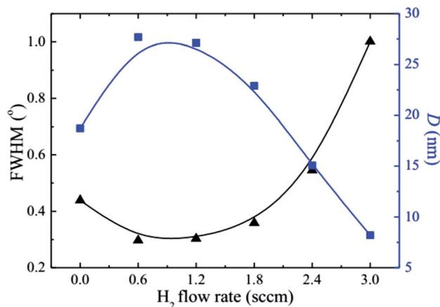
Fig. 3 The FWHM and crystallite size (*D*) of the HNZO films as a function of the flow rate of H<sub>2</sub>.
