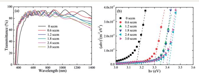
(a) The optical transmittance, and (b) optical band gap of the HNZO films as a function of the flow rate of H<sub>2</sub>.
