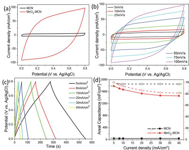
Fig. 5 (a) CV curves of the MCN and  $\text{MnO}_2$ -MCN electrodes obtained using a scanning rate of  $100 \text{ mV s}^{-1}$ ; (b) CV curves of the  $\text{MnO}_2$ -MCN electrode for scanning rates of 5– $100 \text{ mV s}^{-1}$ ; (c) GCD curves of the  $\text{MnO}_2$ -MCN electrode for current densities of 5– $40 \text{ mA cm}^{-2}$ ; and (d) areal capacitance and capacitance retention rate of the MCN and  $\text{MnO}_2$ -MCN electrodes as functions of the current density.
