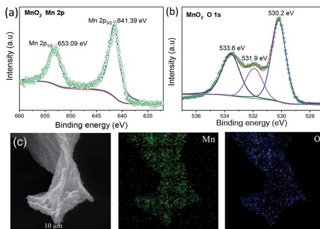
**Fig. 4** XPS spectra and peak fitting of the MnO<sub>2</sub>-MCN electrode (a) Mn and (b) O, and (c) EDS maps of Mn and O for the MnO<sub>2</sub>-MCN electrode.
