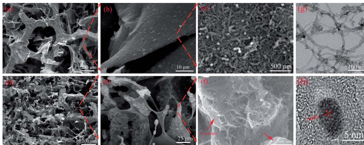
Fig. 2 SEM images of (a–c) MnO<sub>2</sub>-MCN, (d–f) AC-MCN electrodes with different magnifications; and TEM images of (g and h) MnO<sub>2</sub>-MCN electrode with different magnifications.
