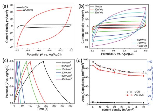
Fig. 6 (a) CV curves of the MCN and AC-MCN electrodes collected at a scanning rate of  $100 \text{ mV s}^{-1}$ ; (b) CV curves of the AC-MCN electrode for scanning rates of 5– $100 \text{ mV s}^{-1}$ ; (c) GCD curves of the AC-MCN electrode for current densities of 5– $40 \text{ mA cm}^{-2}$ ; and (d) areal capacitance and capacitance retention rate of the MCN and AC-MCN electrodes as functions of the current density.
