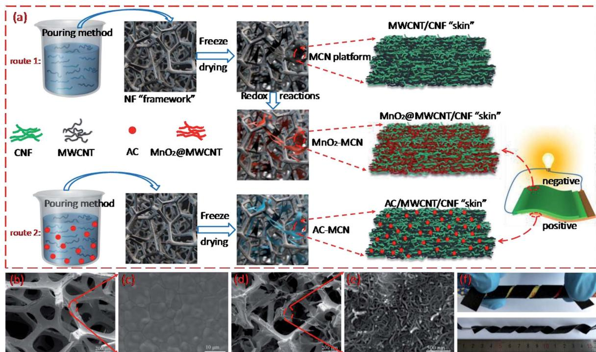
Fig. 1 (a) Illustration of the preparation of the MnO<sub>2</sub>-MCN (route 1) and AC-MCN (route 2) electrodes, and construction of the solid-state ASC device; SEM images of the (b and c) NF and (d and e) MCN hybrid material with different magnifications; and (f) demonstration of the flexibility and bending properties of the MCN electrode sheet.
