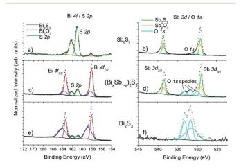
Fig. 6 XPS spectra for  $Sb_2S_3$  (top panels (a) and (b)),  $Bi_2S_3$  (bottom panels (e) and (f)), and  $(Bi_xSb_{1-x})_2S_3$  (middle panels (c) and (d)). The Bi 4f and S 2p spectral regions overlap ((a), (c), (e)), and the Sb 3d region overlaps with O 1s ((b), (d), (f)).
