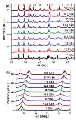
Fig. 3 (a) Powder XRD pattern of  $Bi_2S_3$  bottom,  $(Bi_{1-x}Sb_x)_2S_3$  and  $Sb_2S_3$  top, samples synthesized from different Bi/Sb ratios (b) p-XRD pattern of  $2\theta$  range 27–33 degree showing shift in peaks.
