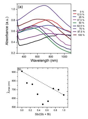
Fig. 10 (a) UV/visible absorption spectrum of  $Bi_2S_3$ ,  $Sb_2S_3$  and  $(Bi_{1-x}-Sb_x)_2S_3$  solid solutions. (b) Plot of absorption maximum against mole fraction of Sb, showing deviation from ideal behaviour.
