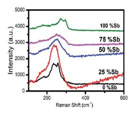
Fig. 11 Raman spectra of nanorods of Sb<sub>2</sub>S<sub>3</sub>, Bi<sub>2</sub>S<sub>3</sub> and  $(Bi_{1-x}Sb_x)_2S_3$  solid solutions.
