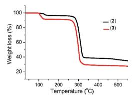
Fig. 1 Thermogram of complexes (2) and (3).
