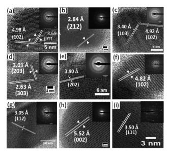
Fig. 5 HRTEM images of synthesized nanorods with Sb/(Sb + Bi) mole fraction of (a) 1:0, (b) 7:1, (c) 3:1, (d) 5:3, (e) 1:1, (f) 3:5, (g) 1:3, (h) 1:7 and (i) 0:1. Inset in each image shows the SAED pattern.
