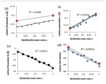
Fig. 4 Variation of lattice constants with increasing mole fraction of Sb obtained from EDS. (a) Lattice parameter a, (b) lattice parameter b, (c) lattice parameter c and (d) cell volume. \* values represent the reported standard value (dotted lines) for  $Bi_2S_3$  and  $Sb_2S_3$ .
