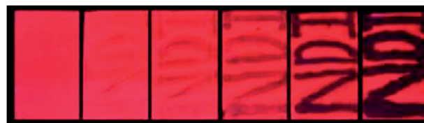
Fig. 5 Images of silica gel plates with copper ions ("NDI" pattern) at different concentrations under a UV-lamp. From left to right, the concentrations of copper ions were 0, 2.0 \times 10^{-6} , 2.0 \times 10^{-5} , 1.0 \times 10^{-4} , 1.0 \times 10^{-3} , and 1.0 \times 10^{-2} mol L -1 .
