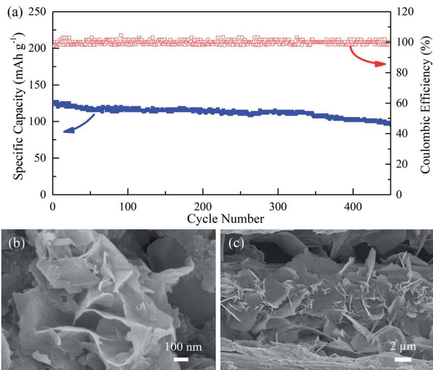
Fig. 3 (a) Cycling stability of the solid-state ZIBs with KCR electrolyte cycled at  $6.0 \text{ A g}^{-1}$  and corresponding coulombic efficiency. SEM images of (b) the  $\text{MnO}_2$  cathode and (c) the electroplated Zn anode after 450 charge/discharge cycles.
