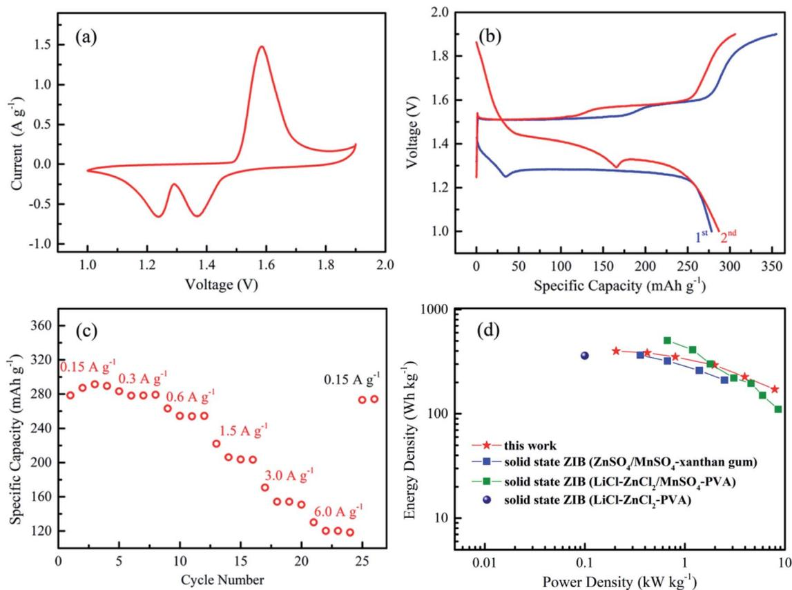
Fig. 2 (a) Cyclic voltammogram of the solid-state ZIBs with KCR electrolyte. (b) The charging/discharging profiles of the first and second cycles at the current density of  $0.15 \text{ A g}^{-1}$ . (c) Specific capacities of the solid-state ZIBs at various current densities. (d) Ragone plots of the solid-state ZIBs with KCR electrolyte. The values reported from other solid-state ZIBs are included for comparison.<sup>13,15,29</sup>
