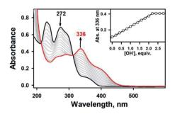
Fig. 5 UV-vis spectral changes showing the formation of 3 (red line) and disappearance of 2a (0.025 mM, black line) upon addition of KOH to 2a in increment of 0.20 equiv. in CH<sub>3</sub>CN at 20 °C. Inset shows the plot of absorbance changes at 336 nm due to 3 (black dot) and against the equivalents of KOH added to 2a in CH<sub>3</sub>CN at 20 °C.
