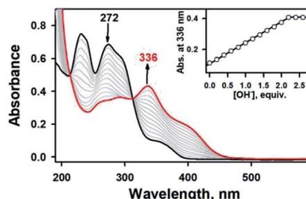
Fig. 5 UV-vis spectral changes showing the formation of **3** (red line) and disappearance of **2a** (0.025 mM, black line) upon addition of KOH to **2a** in increment of 0.20 equiv. in  $\text{CH}_3\text{CN}$  at  $20^\circ\text{C}$ . Inset shows the plot of absorbance changes at 336 nm due to **3** (black dot) and against the equivalents of KOH added to **2a** in  $\text{CH}_3\text{CN}$  at  $20^\circ\text{C}$ .
