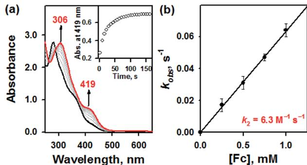
Fig. 3 (a) UV-vis spectra of the reaction of **1a** (0.050 mM) with ferrocene (0.25 mM) in  $\text{CH}_3\text{CN}$  at  $10^\circ\text{C}$ . (b) Plot of pseudo-first-order rate constants ( $k_{\text{obs}}$ ) against the concentrations of ferrocene to determine the  $k_2$  value for **1a** in  $\text{CH}_3\text{CN}$  at  $10^\circ\text{C}$ .
