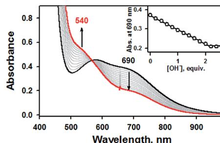
Fig. 2 UV-vis spectral changes showing the formation of **1b** (red line) and disappearance of **1a** (1.0 mM, black line) upon addition of KOH to **1a** in increment of 0.20 equiv. in CH<sub>3</sub>CN at 20 °C. Inset shows the plot of absorbance changes at 690 nm due to **1a** (black dot) and against the equivalents of KOH added to **1a** in CH<sub>3</sub>CN at 20 °C.
