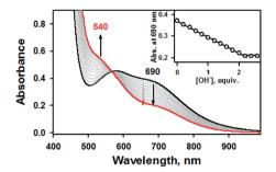
Fig. 2 UV-vis spectral changes showing the formation of 1b (red line) and disappearance of 1a (1.0 mM, black line) upon addition of KOH to 1a in increment of 0.20 equiv. in CH $_3$ CN at 20 °C. Inset shows the plot of absorbance changes at 690 nm due to 1a (black dot) and against the equivalents of KOH added to 1a in CH $_3$ CN at 20 °C.
