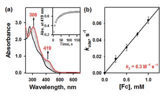
Fig. 3 (a) UV-vis spectra of the reaction of  ${\bf 1a}$  (0.050 mM) with ferrocene (0.25 mM) in CH<sub>3</sub>CN at 10 °C. (b) Plot of pseudo-first-order rate constants ( $k_{\rm obs}$ ) against the concentrations of ferrocene to determine the  $k_2$  value for  ${\bf 1a}$  in CH<sub>3</sub>CN at 10 °C.
