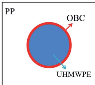
Fig. 5 The core-shell structure of the blends.
