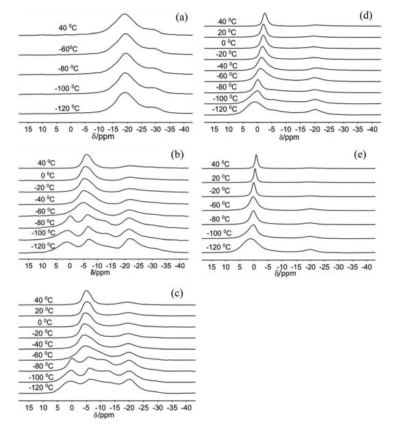
Fig. 1 23Na MAS NMR spectra of Na-hectorite exposed to 0% R.H. (a), 29% R.H. (b), 43% R.H. (c), 70% R.H. (d), and 100% R.H. (e) acquired at the indicated temperatures.
