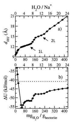
Fig. 3 Computed swelling properties of Na-hectorite with a molar F $^-/$  (F $^-$  + OH $^-$ ) ratio of 0.53 as functions of interlayer H $_2$ O content: (a) basal spacing; (b) hydration energy. The horizontal dashed line in (b) indicates the internal energy of the bulk SPC water model used in the simulations.
