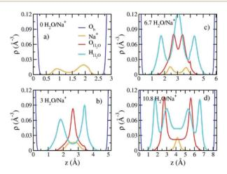
Fig. 4 Computed atomic density profiles (ADPs) as a function of distance normal to the basal hectorite surface (z (Å)) for the indicated interlayer species in Na-hectorite with a molar  $F^-/(F^- + OH^-)$  ratio of 0.53 at the indicated  $H_2O/Na^+$  ratios. (a) collapsed structure; (b) least hydrated monolayer structure; (c) fully hydrated monolayer structure; (d) bilayer structure.
