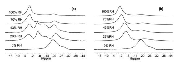
Fig. 2  $^{23}$ Na MAS NMR spectra of Na-hectorite exposed to the indicate R.H.s at -100 °C (a), and 40 °C (b).
