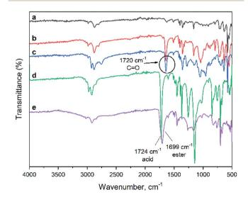
Fig. 2 FTIR spectra of (a) initial and grafted polyHIPEs, (b) polyHIPE-PtBA, (c) polyHIPE-COOH, (d) polyHIPE-PGMA, (e) polyHIPE-NR<sub>2</sub>.
