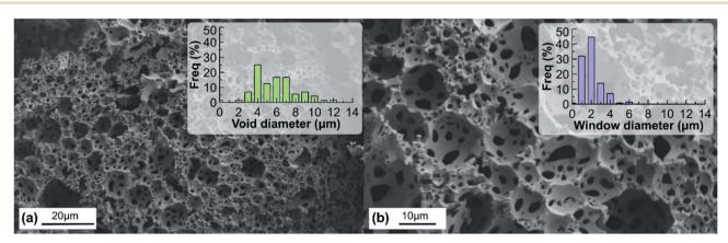
Fig. 1 SEM images of the polyHIPE obtained along with (a) void and (b) window diameter distributions.
