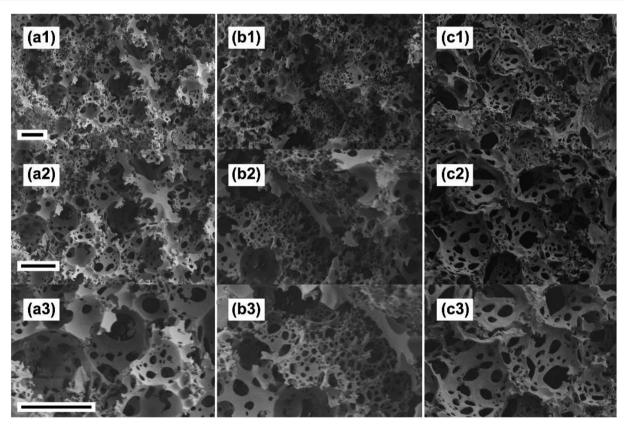
Fig. 5 SEM images of polyHIPE-g-PGMA (a1-a3), polyHIPE-g-PtBA (b1-b3) and catalyst mixture after the reaction (c1-c3). Scale bars are 20 µm.
