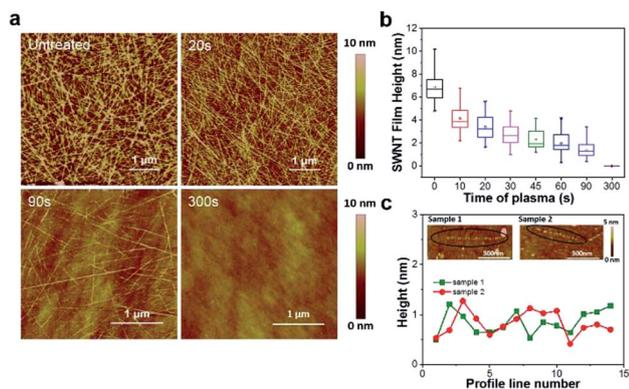
Fig. 3 (a) The AFM images of s-SWNT films treated by plasma etching for different times. The etching time is displayed in the upper left corner of each graph. (b) The height statistics of s-SWNT films with different plasma etching times for 50 profile lines. (c) The AFM images and height statistics of two samples of single s-SWNTs.
