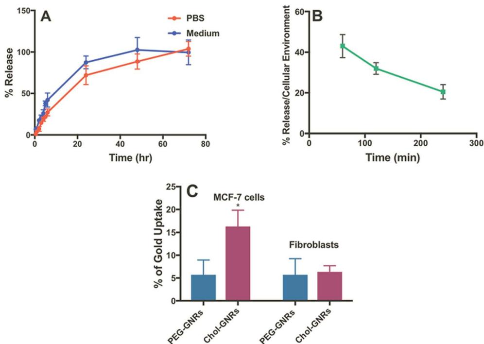
**Fig. 6** *In vitro* release profile of Compound A from the nanocomplex (Chol-A-GNRs) in PBS and in tissue culture medium (A). Release profile of Compound A from the nanocomplex (Chol-A-GNRs) under cellular environment (B). Percentages of cellular uptake of Chol-GNRs and PEG-GNRs into MCF-7 breast cancer cells and human dermal fibroblasts (C). Data are presented as mean  $\pm$  SD,  $n = 3$ . Unpaired *t*-test was used to assess the differences; \* represent  $p < 0.05$ .
