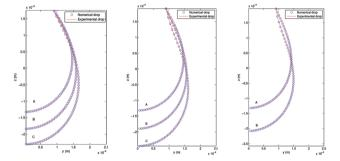
Fig. 5 Experimental and numerical pendant droplets with several volumes: (A)  $V=15~\mu l$ , (B)  $V=20~\mu l$ , (C)  $V=25~\mu l$ . Left: water droplet. Center: gemini surfactant  $4\times 10^{-8}~\text{mol cm}^{-3}$ . Right: gemini surfactant  $1\times 10^{-7}~\text{mol cm}^{-3}$ .
