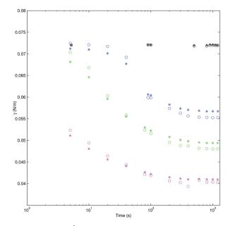
Fig. 7 Tension (N m $^{-1}$ ) of decanol aqueous solution for ADSA (\*) and PRO2TEN (O) at several concentrations *versus* time (s) in log scale: black 0 mol cm $^{-3}$  and air bubble of 40 μl; blue  $4.7 \times 10^{-8}$  mol cm $^{-3}$  and air bubble of 40 μl; green  $8.3 \times 10^{-8}$  mol cm $^{-3}$  and air bubble of 35 μl; magenta  $1.2 \times 10^{-7}$  mol cm $^{-3}$  and air bubble of 20 μl.
