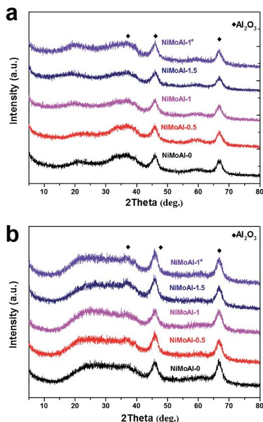
Fig. 3 XRD patterns of the oxide (a) and sulfide (b) NiMoAl- $x$  catalysts.
