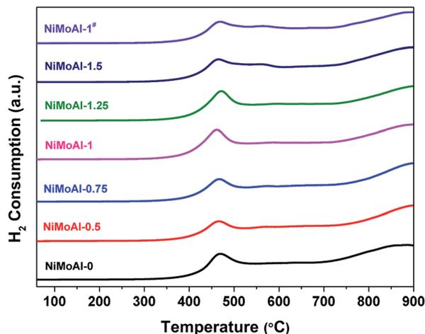
Fig. 4 H<sub>2</sub>-TPR patterns of the oxide catalysts.
