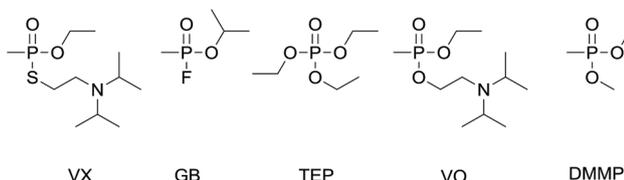
**Fig. 1** The chemical structures of the G and V-series chemical warfare agents VX (2-diisopropylaminoethyl ethyl methylphosphonothiolate) and GB (Sarin, isopropyl methylphosphonofluoridate) and simulants TEP (triethyl phosphate), VO (2-diisopropylaminoethyl ethyl methylphosphonate) and DMMP (dimethyl methylphosphonate) utilised in this investigation.
