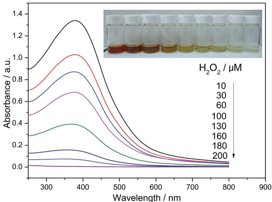
Fig. 3 UV-vis absorption spectra of  $\text{MnO}_2$  solution upon the addition of  $\text{H}_2\text{O}_2$  solution with various concentrations. The inset shows the corresponding photographs of the reaction solution.
