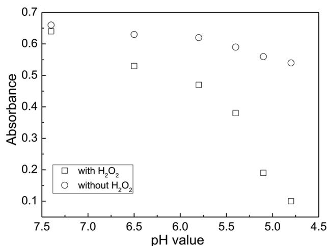
Fig. 2 A comparison of the MnO<sub>2</sub> solution absorbance with and without the addition of H<sub>2</sub>O<sub>2</sub> under the reaction conditions with different pH values. The reaction time was fixed at 3 min.
