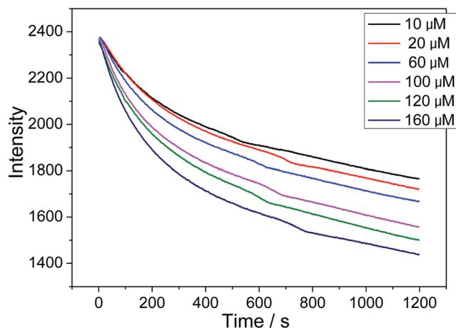
Fig. 4 Time and  $\text{H}_2\text{O}_2$  concentration dependent luminescence response of  $[\text{Ru}(\text{dpp})_3]\text{Cl}_2$  under 535 nm excitation.
