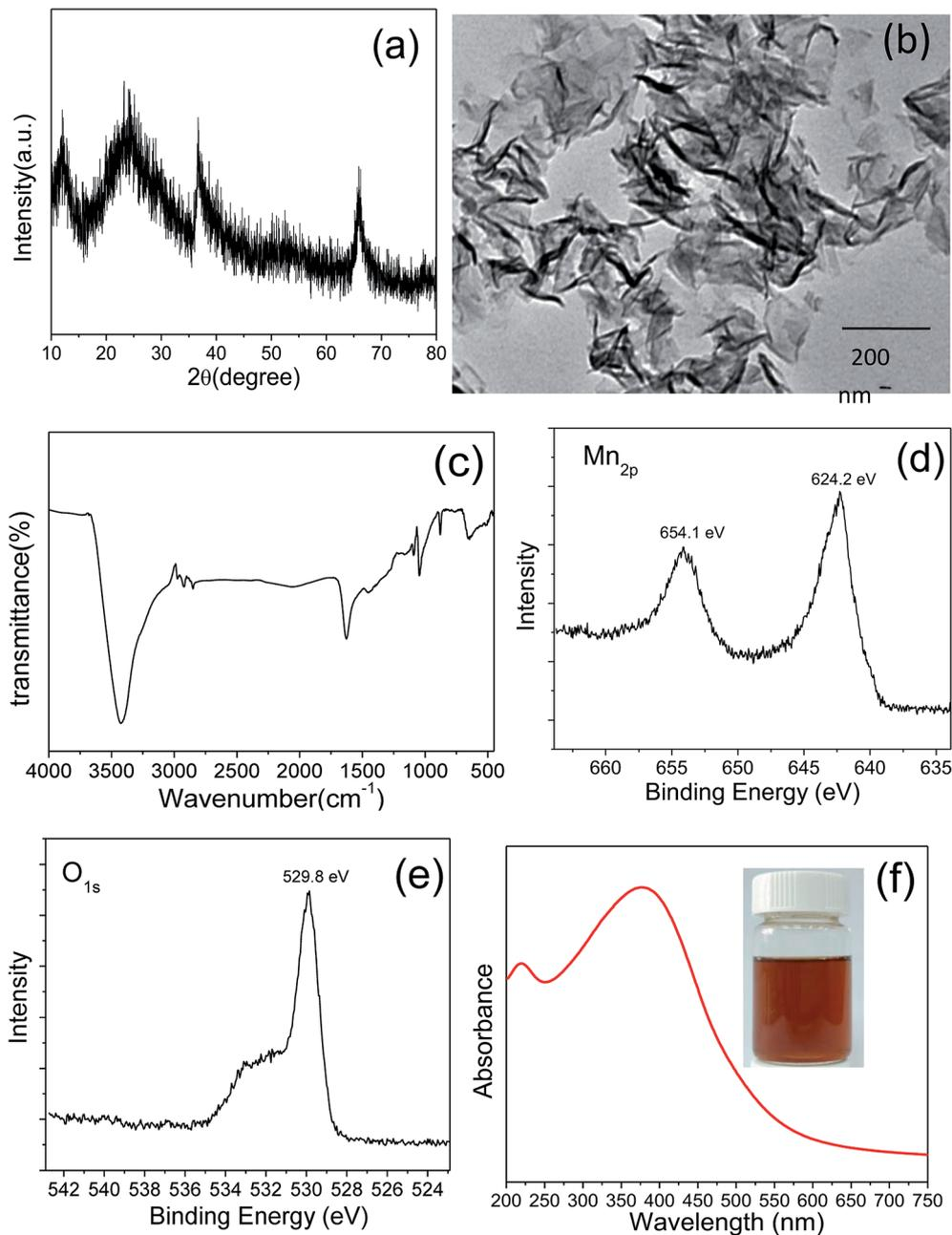
Fig. 1 XRD pattern (a), TEM image (b), FT-IR spectrum (c), XPS spectra of  $\text{Mn}_{2p}$  (d) and  $\text{O}_{1s}$  (e), and UV-vis absorption spectrum (f) of the synthesized  $\text{MnO}_2$  nanosheets.
