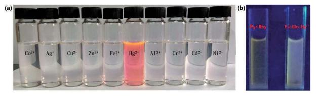
Fig. 4 (a) Colorimetric performance of sensor Pyr-Rhy (10  $\mu$ M) upon addition of different metal ions (1.0 equiv.) in DMSO/H<sub>2</sub>O (1/1, v/v) solution; (b) color change induced upon addition of Hg<sup>2+</sup> under 365 nm UV lamp.
