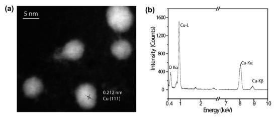
Fig. 4 (a) Selected HAADF-STEM image of CuNP and (b) STEM-EDS profile of CuNP.
