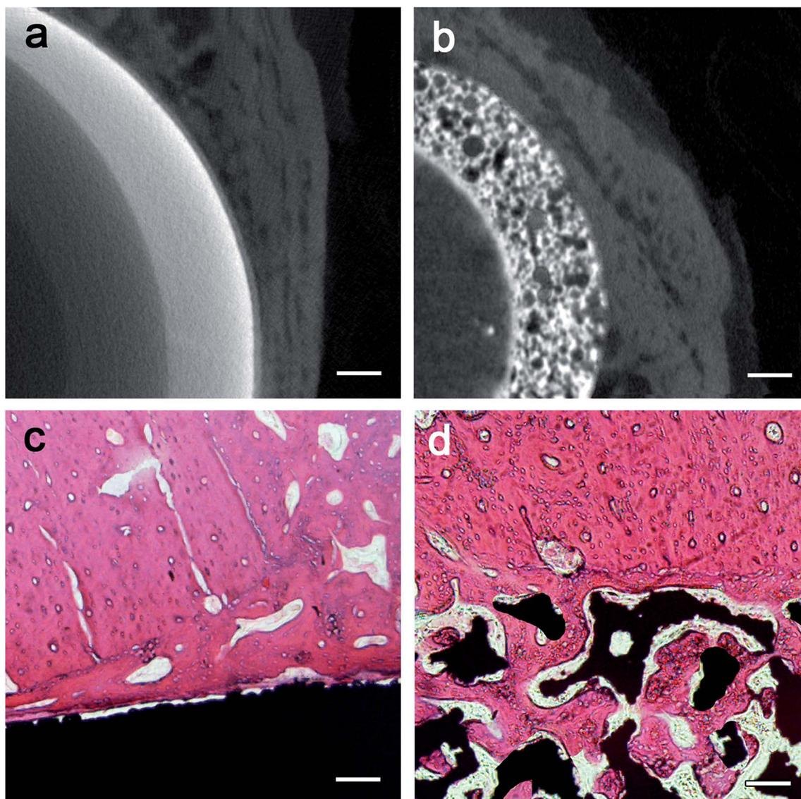
**Fig. 6** Micro-CT images of (a) the HA-coated cup and (b) the fully porous Ti6Al4V after one-year implantations. The scale bar in each image represents 2 mm. And histopathologic images of (c) the HA-coated cup and (d) the fully porous Ti6Al4V after one-year implantations. The scale bar in each image represents 200  $\mu\text{m}$ .
