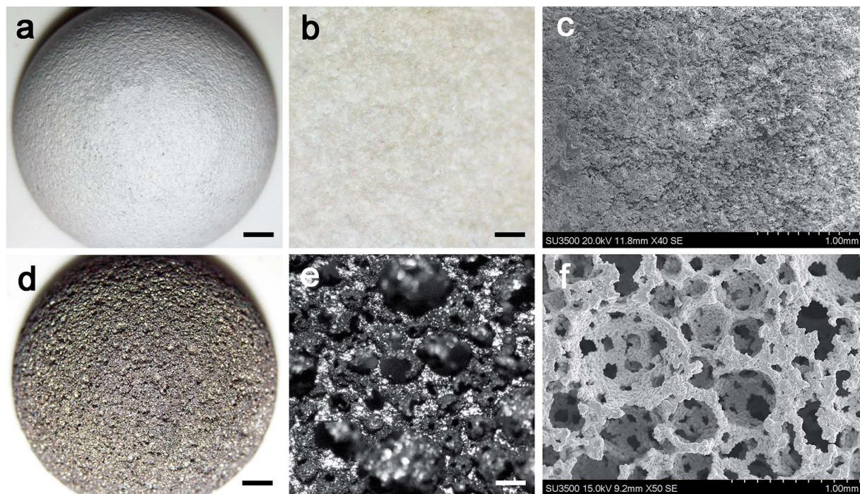
**Fig. 3** Characterization of (a–c) HA-coated and (d–f) fully porous acetabular cup: (a) and (d) are optical microscope images with ×1 magnification, the scale bar represents 2 mm; (b) and (e) are optical microscope images with ×5 magnification, the scale bar represents 500 μm; (c) and (f) are SEM images, the scale bar represents 1 mm.
