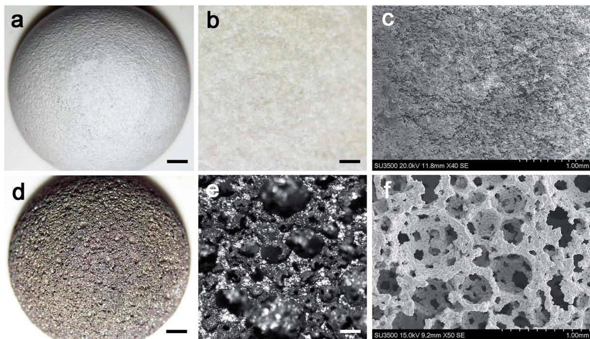
**Fig. 3** Characterization of (a–c) HA-coated and (d–f) fully porous acetabular cup: (a) and (d) are optical microscope images with ×1 magnification, the scale bar represents 2 mm; (b) and (e) are optical microscope images with ×5 magnification, the scale bar represents 500 µm; (c) and (f) are SEM images, the scale bar represents 1 mm.
