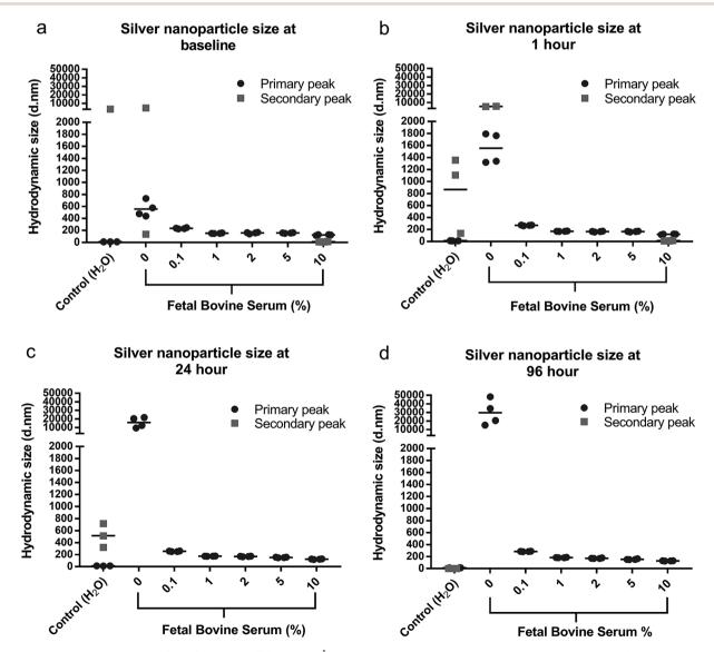
Fig. 2 Hydrodynamic particle size (d nm) of AgNPs (22.5  $\mu$ g ml<sup>-1</sup>) dispersed in either DMEM with increasing Fetal Bovine Serum concentration measured at 0, 1, 24, and 96 h using dynamic light scattering.
