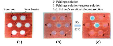
Fig. 6 The fabricated  $\mu$ PAD for the detection of glucose using Fehling's solution: (a)  $\mu$ PAD after wax printing and laser-induced penetration; (b) Fehling's solution, sucrose solution and glucose solution were added to the reservoirs using a pipette; (c) a chromogenic reaction occurred between Fehling's solution and glucose (in brick-red) in reservoirs 2 to 6.
