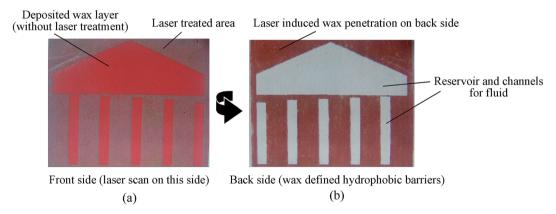
Fig. 3 Front and back sides showing the laser-induced penetration of the paper-based microfluidic devices: (a) front side after diode laser scan; (b) back side after diode laser scan.
