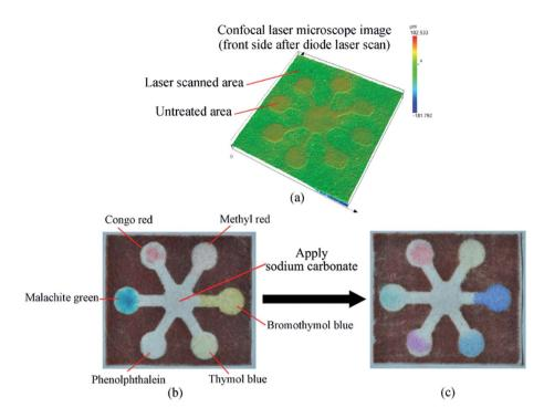
Fig. 5 The fabricated  $\mu$ PAD for pH tests: (a) the laser confocal microscope image for the laser scanned pattern on the front side of the filter paper; (b) the application of various reaction reagents for the pH test; (c) the color-change reactions on  $\mu$ PAD after applying sodium carbonate.
