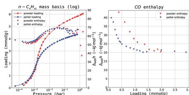
Fig. 5 Selected isotherms from the MIL-127(Fe) dataset: (left) C<sub>4</sub>H<sub>10</sub> adsorption isotherms and (right) CO enthalpy curves. Results are in red for the powder and blue for the shaped samples.
