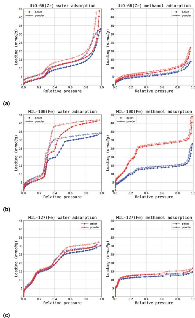
Fig. 7 Water (left) and methanol (right) adsorption isotherms (a) UiO-66(Zr), (b) MIL-100(Fe) and (c) MIL-127(Fe). The powder and  $\rho$ -alumina isotherms are displayed in red and dark blue respectively.
