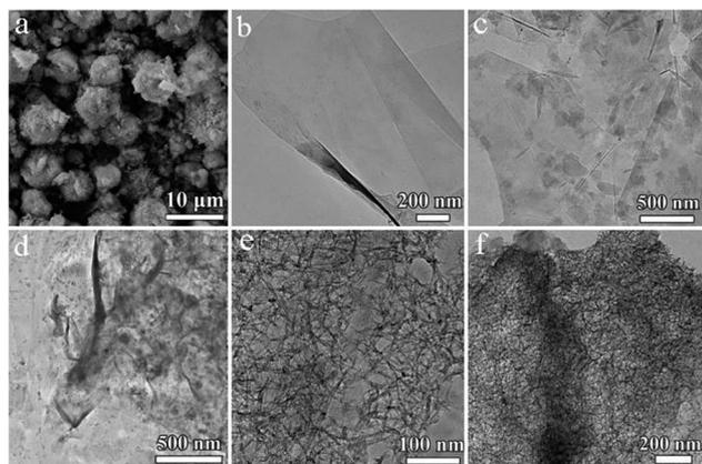
**Fig. 1** (a) SEM image of NiAl-LDH; TEM images of (b) pure EG; (c) EG/NA1 composite synthesized in the presence of EG and with a low loading of urea (0.5 mmol); (d) EG/NA2 composite synthesized with an intermediate loading of urea (1 mmol); (e and f) EG/NA3 and EG/NA4 nanowires synthesized with high loadings of urea (2 mmol and 3 mmol).
