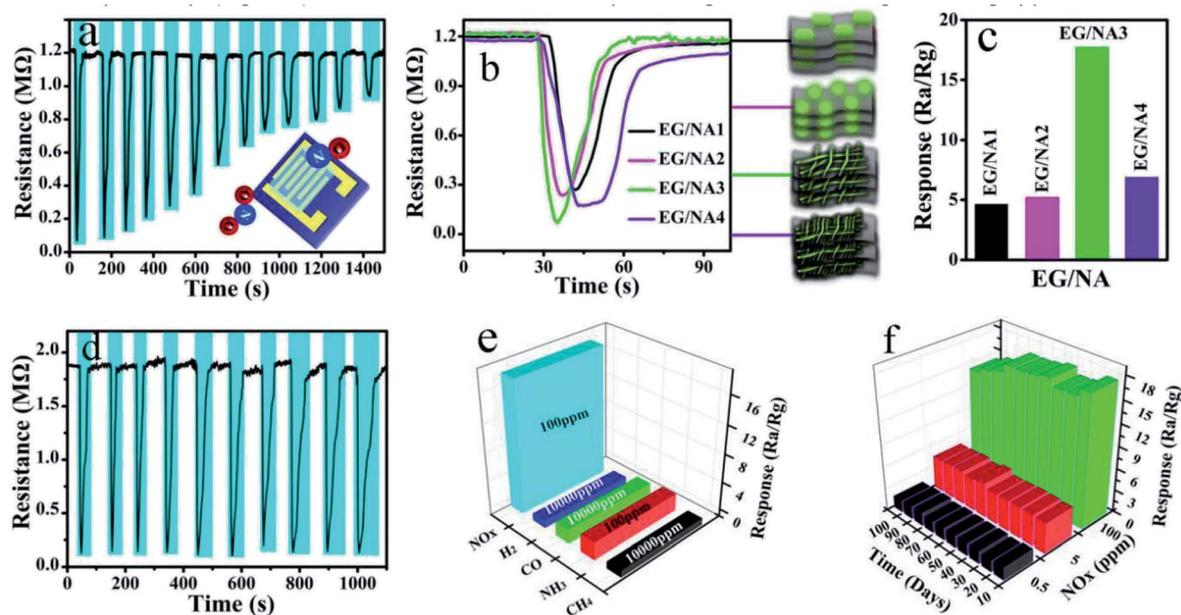
Fig. 5 (a) The transient dynamical responses of the EG/NA3 composite to different concentrations of 100–0.01 ppm NO<sub>x</sub>; (b and c) responses of the EG/NA sensors to 100 ppm NO<sub>x</sub>; (d) reproducibility of the EG/NA3 sensor on successive exposure (10 cycles) to 100 ppm NO<sub>x</sub>; (e) the selectivity for various gases; (f) the response of EG/NA3 for 100 days with 100, 5, and 0.5 ppm NO<sub>x</sub> at RT (24 ± 2 °C).
