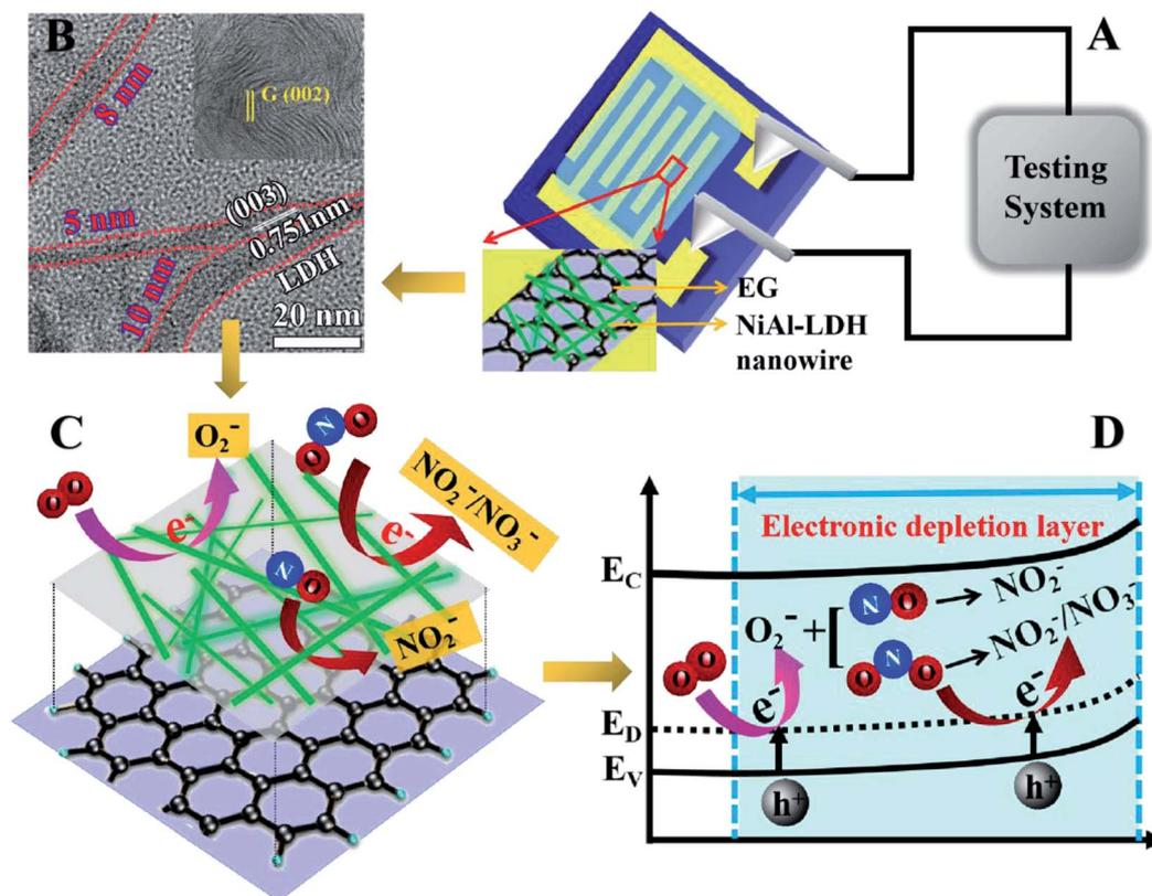
**Scheme 2** The scheme of the proposed gas sensing mechanism: (A) test device diagram; (B) HRTEM image of EG/NA3; (C) sketch of the EG/NA3 sensor exposed to  $\text{NO}_x$  ( $\text{NO}$  and  $\text{NO}_2$ ); (D) oxygen molecules trap electrons to form chemisorbed oxygen and give  $\text{NO}_x$  gas sensing response.
