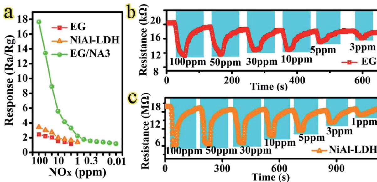
Fig. 6 (a) Responses of EG, NiAl-LDH and EG/NA3 composites to different concentrations of NO<sub>x</sub> at RT (24 ± 2 °C); (b and c) transient dynamical responses of EG and NiAl-LDH, respectively, to different concentrations of NO<sub>x</sub>.
