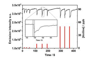
Fig. 3 Time-resolved fluorescence intensity (black line) of a PDI@PVDF fibril film upon consecutive exposures to various concentrations of aniline vapors. (1 s exposures, concentrations indicated by the red columns). Inset: fluorescence change upon exposure to 10 ppb aniline, and the filled rectangle indicated the exposure times (the emission intensity at 630 nm was measured for every 300 ms,  $\lambda_{ex} = 365$  nm).
