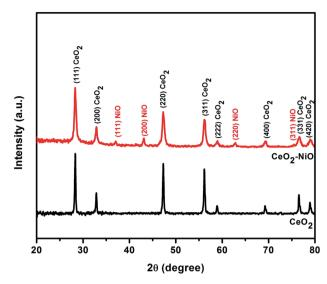
Fig. 2 XRD patterns of pure  ${\rm CeO_2}$  nanoparticles and  ${\rm NiO/CeO_2}$  nanocomposites.
