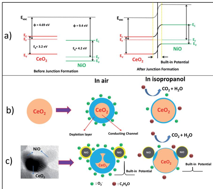
Fig. 10 (a) Schematic diagram demonstrating the band gap alignment of NiO/CeO<sub>2</sub>. Schematic illustration of the isopropanol gas sensing mechanism of (b) CeO<sub>2</sub> and (c) NiO/CeO<sub>2</sub> gas sensors with surface adsorption and desorption reactions.
