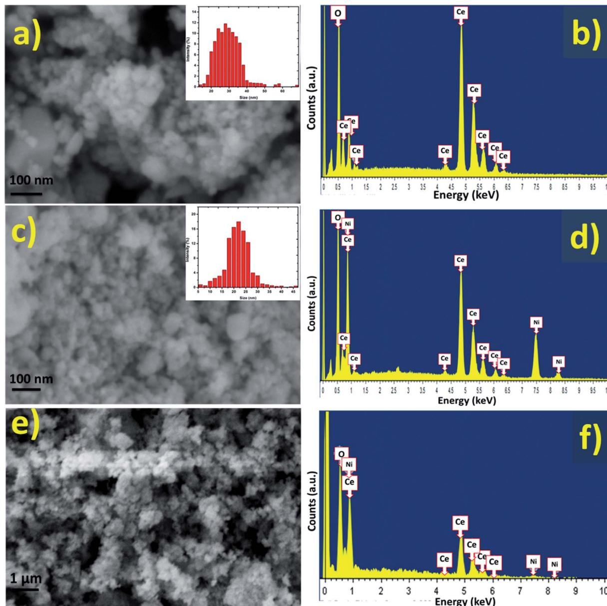
Fig. 4 FESEM images of (a)  $\text{CeO}_2$  nanoparticles, (c)  $\text{NiO/CeO}_2$  nanocomposites. EDS spectra of (b) pure  $\text{CeO}_2$  nanoparticles, and (d)  $\text{NiO/CeO}_2$  nanocomposites. (e) SEM micrographs and (f) EDS spectrum of fabricated gas sensor using  $\text{NiO/CeO}_2$  nanocomposites. Insets are the particle size distributions.
