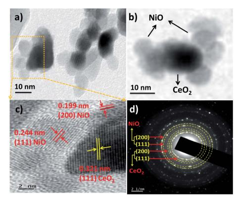
Fig. 5 (a and b) HRTEM images of NiO/CeO<sub>2</sub> nanocomposites with different magnifications. (c) *d*-spacing and (d) SAED pattern of NiO/CeO<sub>2</sub> nanocomposites.
