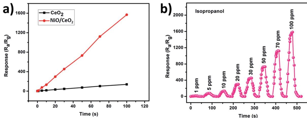
Fig. 7 (a) Response of CeO<sub>2</sub> and NiO/CeO<sub>2</sub> gas sensors towards various concentrations of isopropanol gas at room temperature. (b) Dynamic response and recovery curves of NiO/CeO<sub>2</sub> gas sensor towards isopropanol gas at room temperature.
