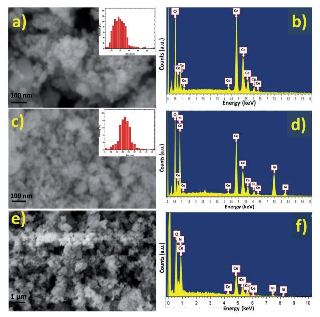
Fig. 4 FESEM images of (a) CeO<sub>2</sub> nanoparticles, (c) NiO/CeO<sub>2</sub> nanocomposites. EDS spectra of (b) pure CeO<sub>2</sub> nanoparticles, and (d) NiO/CeO<sub>2</sub> nanocomposites. (e) SEM micrographs and (f) EDS spectrum of fabricated gas sensor using NiO/CeO<sub>2</sub> nanocomposites. Insets are the particle size distributions.
