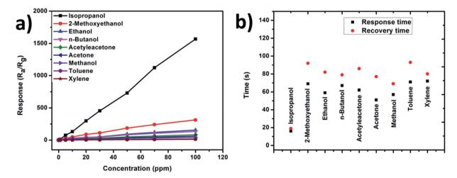
Fig. 8 (a) Response of NiO/CeO<sub>2</sub> gas sensor versus varying concentrations (1–100 ppm) of test gases at room temperature. (b) Response and recovery times of NiO/CeO<sub>2</sub> gas sensor towards 100 ppm test gases at room temperature.
