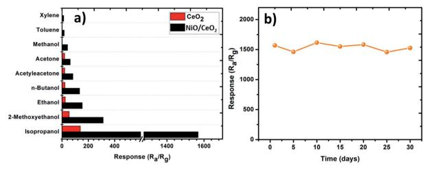
Fig. 9 (a) Response of  $CeO_2$ , and  $NiO/CeO_2$  gas sensors towards 100 ppm test gases at room temperature. (b) The long-term stability of  $NiO/CeO_2$  gas sensor towards 100 ppm isopropanol at room temperature.
