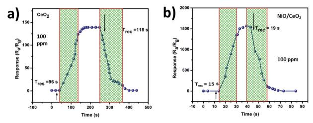
Fig. 6 Response and recovery of (a) CeO<sub>2</sub>, and (b) NiO/CeO<sub>2</sub> gas sensors towards 100 ppm isopropanol gas at room temperature.
