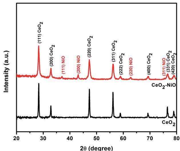
Fig. 2 XRD patterns of pure  $\text{CeO}_2$  nanoparticles and  $\text{NiO/CeO}_2$  nanocomposites.
