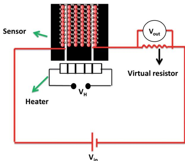
Fig. 1 Schematic representation of gas sensing measurement circuit.
