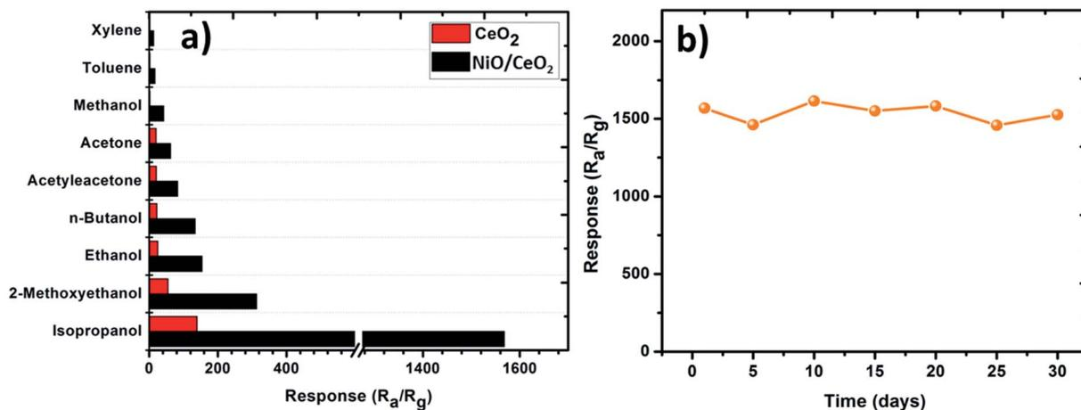
Fig. 9 (a) Response of CeO<sub>2</sub> and NiO/CeO<sub>2</sub> gas sensors towards 100 ppm test gases at room temperature. (b) The long-term stability of NiO/CeO<sub>2</sub> gas sensor towards 100 ppm isopropanol at room temperature.
