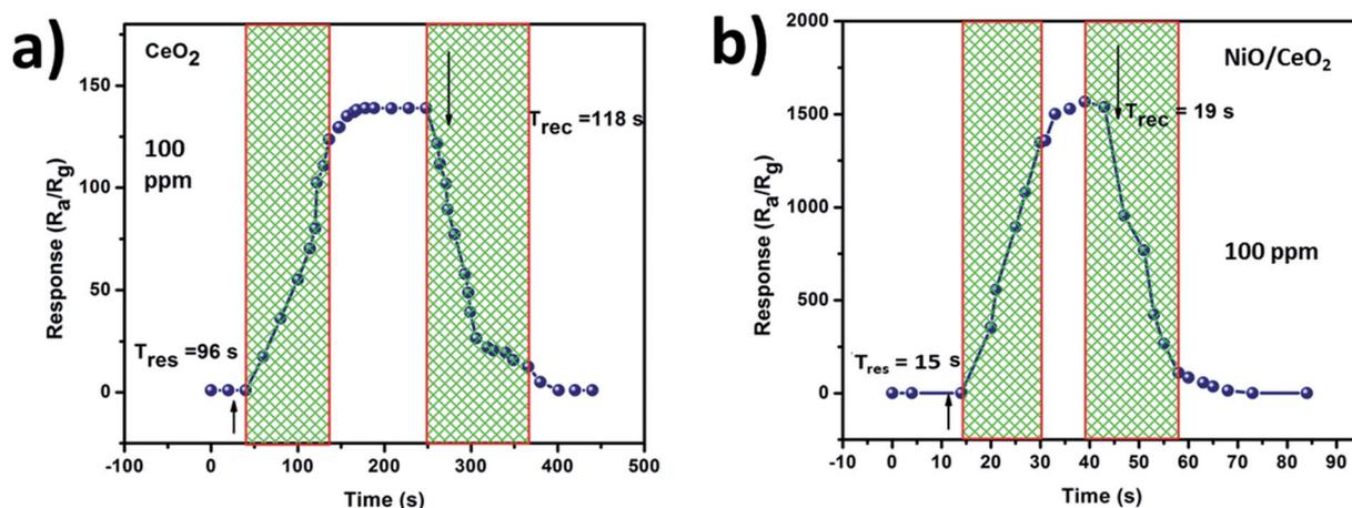
Fig. 6 Response and recovery of (a) CeO<sub>2</sub>, and (b) NiO/CeO<sub>2</sub> gas sensors towards 100 ppm isopropanol gas at room temperature.
