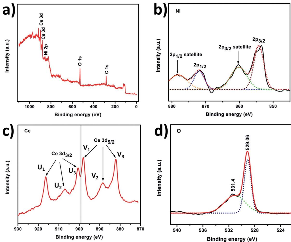
Fig. 3 XPS spectra of (a) NiO/CeO<sub>2</sub>, (b) Ni 2p and (c) Ce 3d, and (d) O 1s.
