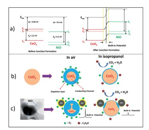
Fig. 10 (a) Schematic diagram demonstrating the band gap alignment of NiO/CeO2. Schematic illustration of the isopropanol gas sensing mechanism of (b) CeO<sub>2</sub> and (c) NiO/CeO<sub>2</sub> gas sensors with surface adsorption and desorption reactions.
