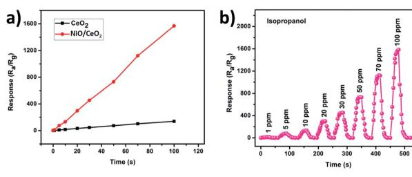
Fig. 7 (a) Response of CeO<sub>2</sub>, and NiO/CeO<sub>2</sub> gas sensors towards various concentrations of isopropanol gas at room temperature. (b) Dynamic response and recovery curves of NiO/CeO<sub>2</sub> gas sensor towards isopropanol gas at room temperature.
