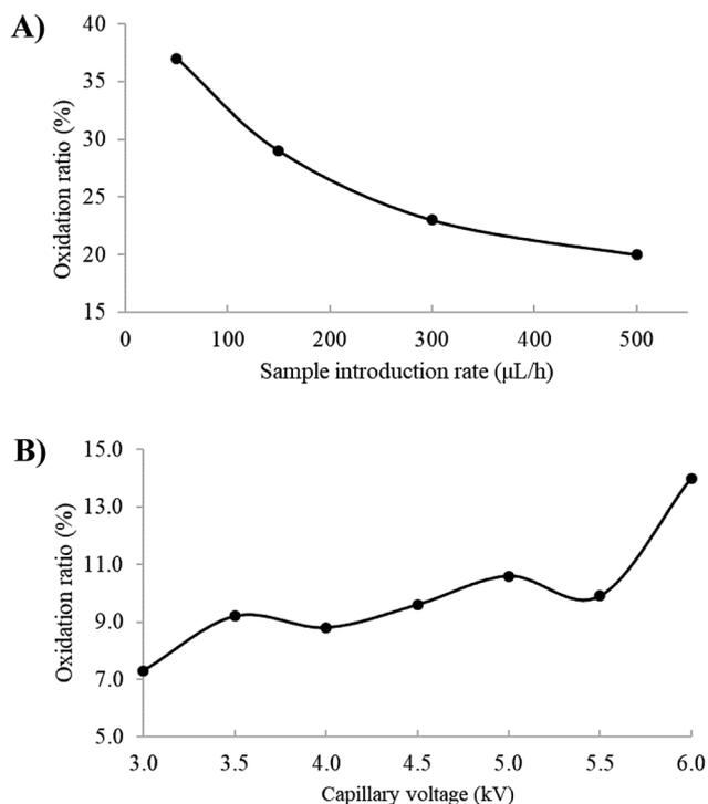
Fig. 2 When methanol was used as the solvent, plot of oxidation ratio (%) of compound **1** versus (A) sample introduction rate over the range from 50–500  $\mu\text{L h}^{-1}$ ; (B) capillary voltage from 3.0 to 6.0 kV. Oxidation ratio (%) =  $(I_{[M-H]^+} + I_{[M]^{2+}}) / (I_{[M-H]^+} + I_{[M]^{2+}} + I_{[M+H]^+} + I_{[M+Na]^+} + I_{[M+K]^+}) \times 100\%$ .
