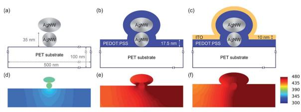
Fig. 4 (a)–(c) Schematic illustration and specification of the cross-section of the AgNW, AgNW–PEDOT:PSS, and AgNW–PEDOT:PSS/ITO films in the device simulation, and (d)–(f) the resulting temperature distribution when the maximum temperature reaches  $T_{\rm m}$ . Note that the detailed position of the cross-section is depicted in Fig. S1 in ESI.†
