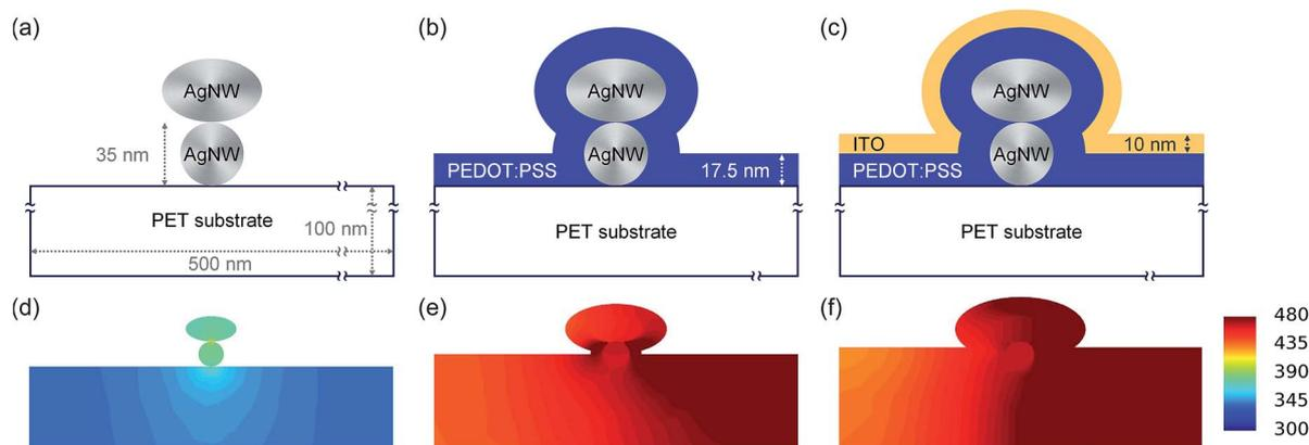
Fig. 4 (a)–(c) Schematic illustration and specification of the cross-section of the AgNW, AgNW–PEDOT:PSS, and AgNW–PEDOT:PSS/ITO films in the device simulation, and (d)–(f) the resulting temperature distribution when the maximum temperature reaches  $T_m$ . Note that the detailed position of the cross-section is depicted in Fig. S1 in ESI†
