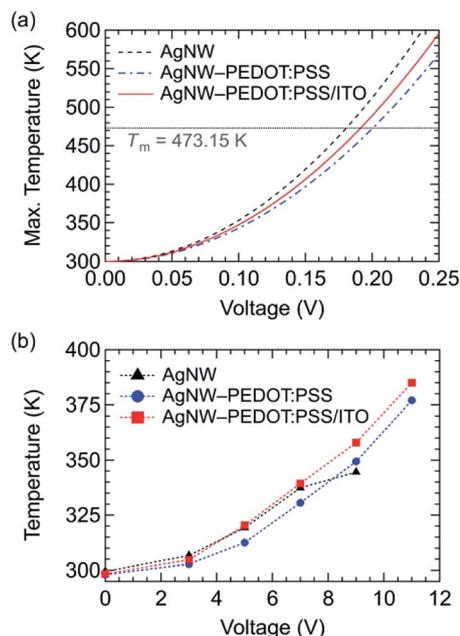
Fig. 3 (a) Simulated maximum temperature within the films by the joule heating in the AgNW, AgNW–PEDOT:PSS, and AgNW–PEDOT:PSS/ITO films. The melting point of the AgNW ( $T_m$ ) is indicated. (b) Experimental data of the mean temperature in the flexible TFHs over the bias voltages.
