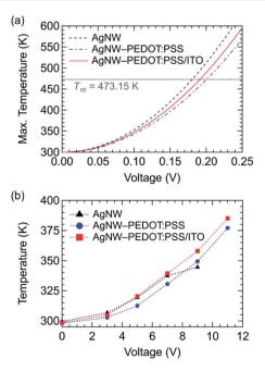
Fig. 3 (a) Simulated maximum temperature within the films by the joule heating in the AgNW, AgNW-PEDOT:PSS, and AgNW-PEDOT:PSS/ITO films. The melting point of the AgNW ( $T_{\rm m}$ ) is indicated. (b) Experimental data of the mean temperature in the flexible TFHs over the bias voltages.
