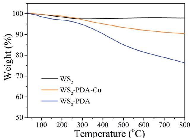
Fig. 2 TGA thermograms of WS<sub>2</sub>, WS<sub>2</sub>-PDA and WS<sub>2</sub>-PDA-Cu.
