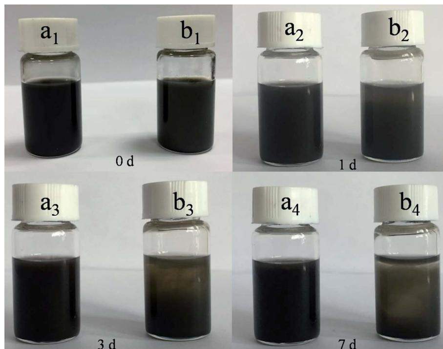
Fig. 5 Dispersion of WS<sub>2</sub>-PDA-Cu (a<sub>1</sub>-a<sub>4</sub>) and WS<sub>2</sub>-Cu (b<sub>1</sub>-b<sub>4</sub>) in PAG base oil.
