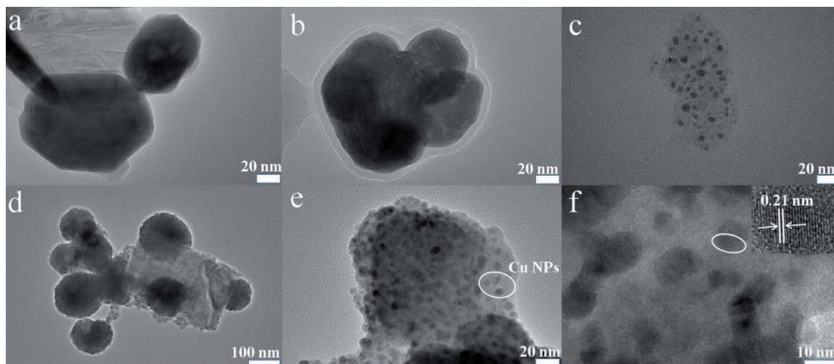
Fig. 4 TEM images of  $WS_2$  (a),  $WS_2$ -PDA (b), Cu NPs (c),  $WS_2$ -Cu (d) and  $WS_2$ -PDA-Cu (e and f).
