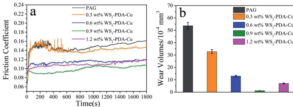
Fig. 7 Friction coefficient (a) and wear volume (b) of the discs lubricated by PAG containing WS<sub>2</sub>-PDA-Cu with different concentrations (load, 100 N; temperature, 150 °C; stroke, 1 mm; frequency, 25 Hz).
