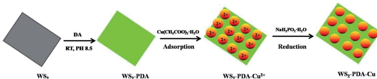
Scheme 1 Schematic of synthetic WS<sub>2</sub>-PDA-Cu.
