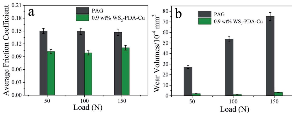
Fig. 8 Average friction coefficient and wear volume of the discs lubricated by PAG and PAG containing 0.9 wt% WS<sub>2</sub>-PDA-Cu under various loads (temperature, 150 °C; stroke, 1 mm; frequency, 25 Hz).
