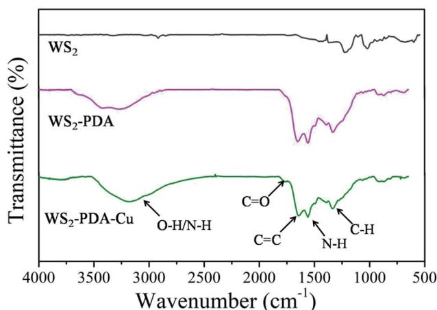
Fig. 1 The FTIR spectra of WS<sub>2</sub>, WS<sub>2</sub>-PDA and WS<sub>2</sub>-PDA-Cu.
