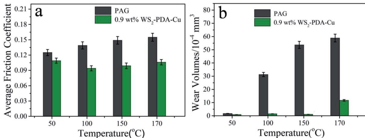
Fig. 9 Average friction coefficient and wear volume of the discs lubricated by PAG and PAG containing 0.9 wt% WS<sub>2</sub>-PDA-Cu at various temperature (load, 100 N; stroke, 1 mm; frequency, 25 Hz).
