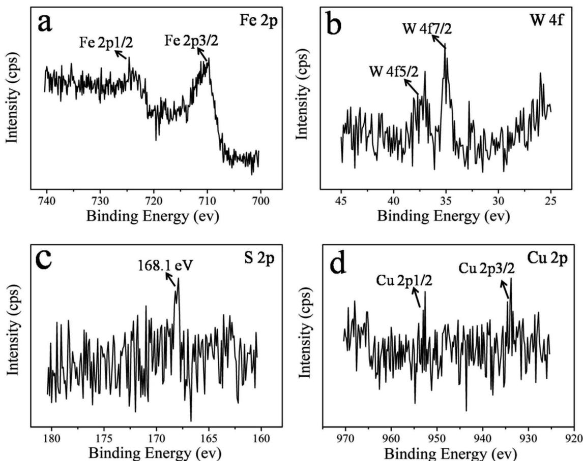
Fig. 11 XPS spectra of wear surfaces on the discs lubricated by PAG containing WS<sub>2</sub>-PDA-Cu (load, 100 N; temperature, 150 °C; stroke, 1 mm; frequency, 25 Hz), Fe 2p (a), W 4f (b), S 2p (c) and Cu 2p (d).
