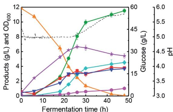
Fig. 6 The time courses of butanol fermentation with five phenolics addition ( $0.2\text{ g L}^{-1}$ ) under the pH-control strategy. ●: butanol; ◆: acetone; ●: ethanol; ■: acetate; ▼: butyrate; ★:  $\text{OD}_{600}$ ; ▲: glucose; broken line: pH. The adding amount of phenolics was  $0.04\text{ g L}^{-1}$  vanillin,  $0.04\text{ g L}^{-1}$  vanillic acid,  $0.04\text{ g L}^{-1}$  *p*-hydroxybenzaldehyde,  $0.04\text{ g L}^{-1}$  *p*-hydroxybenzoic acid, and  $0.04\text{ g L}^{-1}$  ferulic acid.
