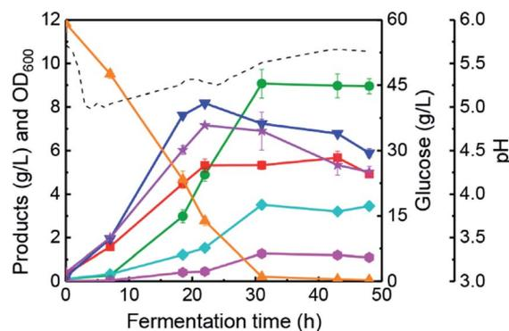
Fig. 4 The time courses of butanol fermentation with vanillin (0.1 g L<sup>-1</sup>) and vanillic acid (0.1 g L<sup>-1</sup>) addition under the pH-control strategy. ●: butanol; ◆: acetone; ●: ethanol; ■: acetate; ▼: butyrate; ★: OD<sub>600</sub>; ▲: glucose; broken line: pH.
