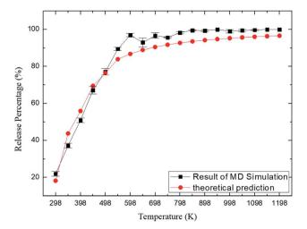
Fig. 5 Release percentage of methane as a function of temperature. Squares and circles are the results of MD simulations and theoretical predictions, respectively.
