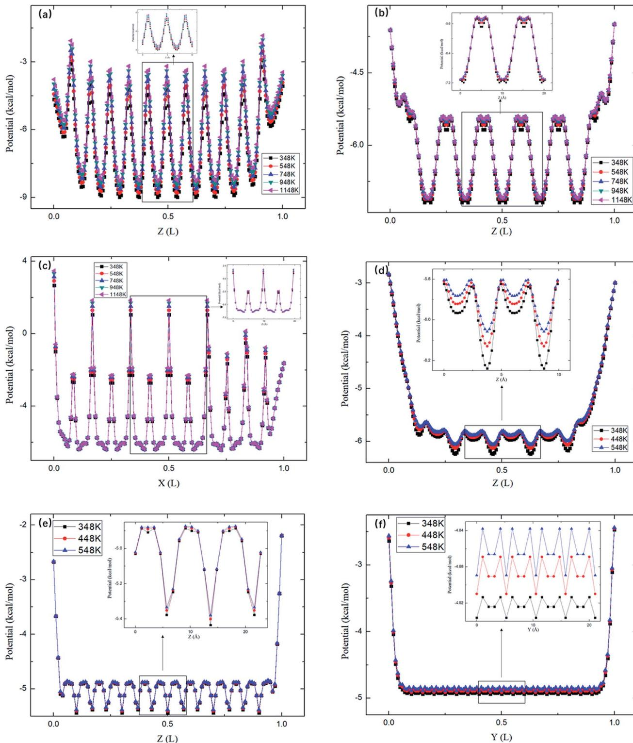
Fig. 8 The average potential profile of zeolite structures in Table 2. (a) ABW. (b) Straight channels of TER. (c) Zigzag channels of TER. (d) VET. (e) OFF. (f) CFI, where  $L$  is the length of the corresponding channel.
