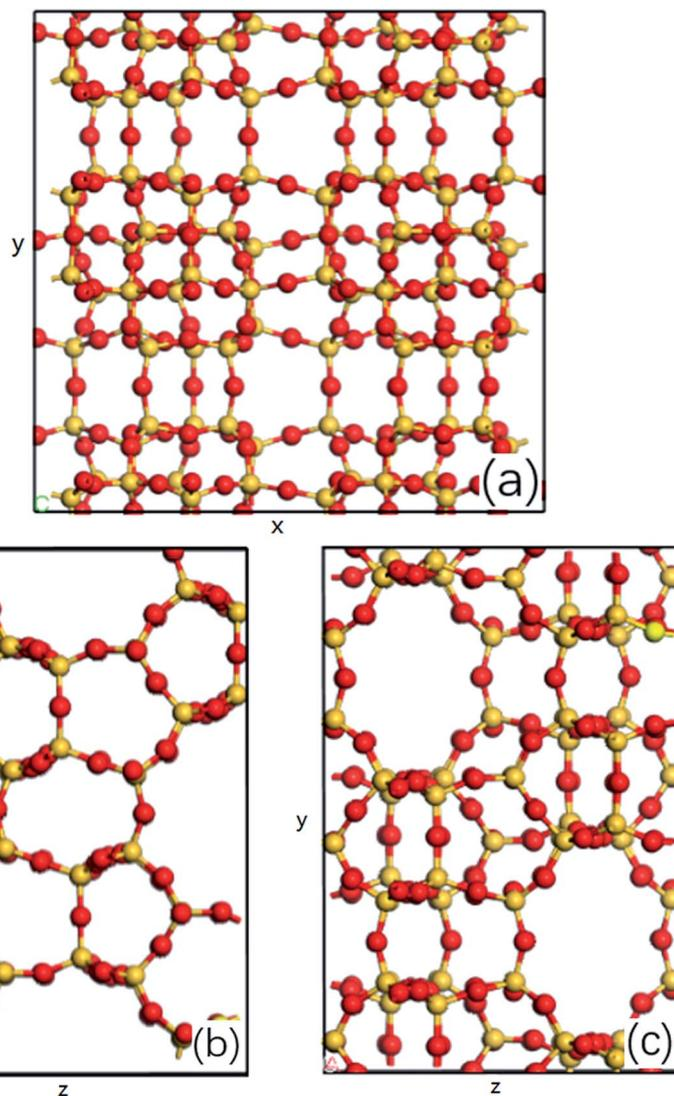
Fig. 2 (a) Main view, (b) top view and (c) left view of all-silica MFI zeolite structure, silicon atoms are represented by the yellow balls and oxygen atoms are represented by the red balls,  $x$ ,  $y$  and  $z$  represent the edges of a unit cell in  $x$ ,  $y$  and  $z$  direction.
