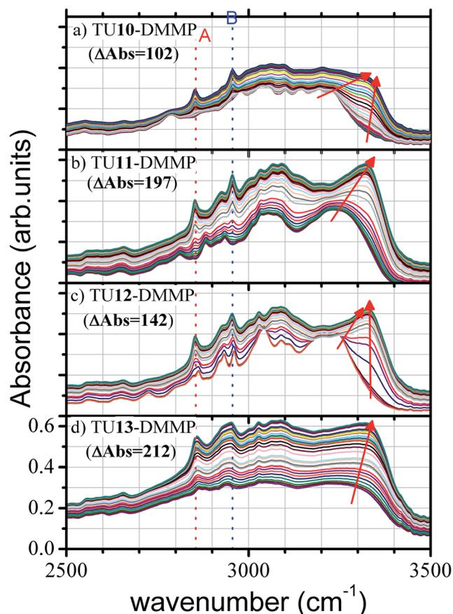
Fig. 2 Diffuse reflectance IR spectra of TU $n$  ( $n = 10$ – $13$ ) during the DMMP adsorption process. Each spectral window consists of a sequence of 37 spectra recorded with 5 min interval starting from 30 s after dosing DMMP. The values denoted with  $\Delta$ Abs are the differences in the integrated intensities between the last spectrum and the first spectrum.
