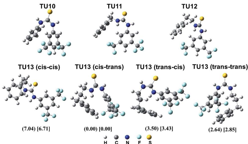
Fig. 3 Geometries of global minimum conformers of TUn ( $n = 10-12$ ) and four lowest energy conformers for the four isomers of TU13. For the four isomers of TU13, the relative values of  $E_e$  and  $E_o$  in kcal mol<sup>-1</sup> are shown in parentheses and square brackets, respectively.
