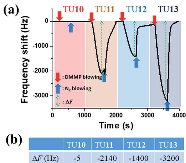
Fig. 1 The QCM response curves for TUn (n = 10–13) receptors (a) and the table for the corresponding  $\Delta F$  values (b). The DMMP concentration was 60 ppm.
